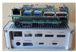
Fig. 1: Thunderbolt dock with FPGA implant, an implementation of our I/O-security research platform
