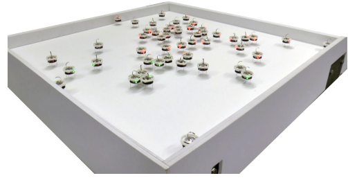
Fig. 3. We tested the most resilient methods on a swarm of 50 Kilobots with 5 contrarians.
