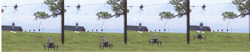
Fig. 1: Snapshots depicting a multirotor docking with a suspended platform outdoors. Our outdoor setup comprises of pulleys interconnected by an actuated “zipline” mechanism to regulate the translational velocity of the platform suspended from it.
