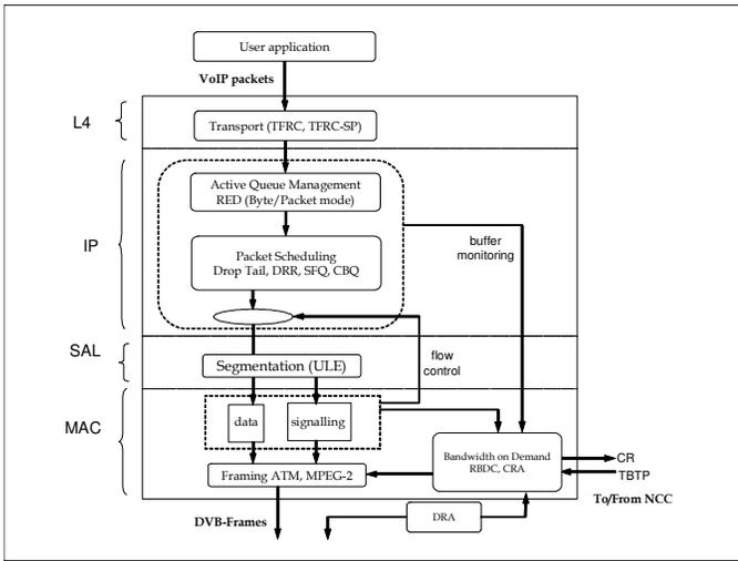
Figure 1 RCST access gateway networking diagram
