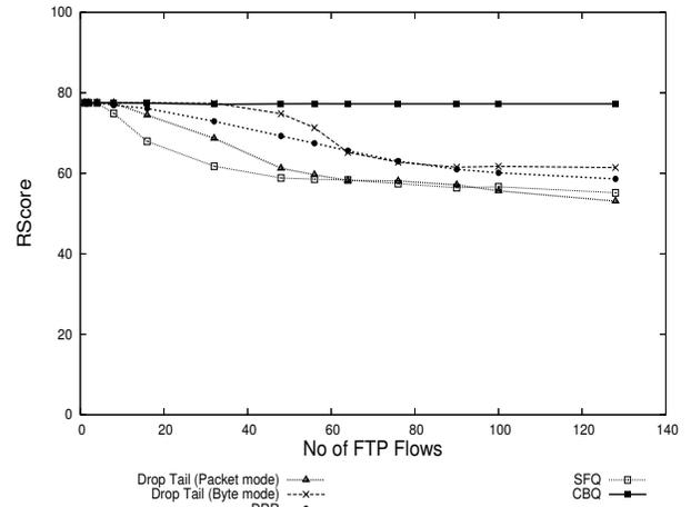
Figure 5 R-score of VoIP flows for different scheduling mechanisms.
