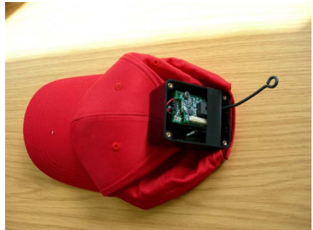
Figure 3: A MICA2 mote [6] with MTS310 sensor board [7] attached to a baseball hat. These are worn by players of Trove, during the game.
