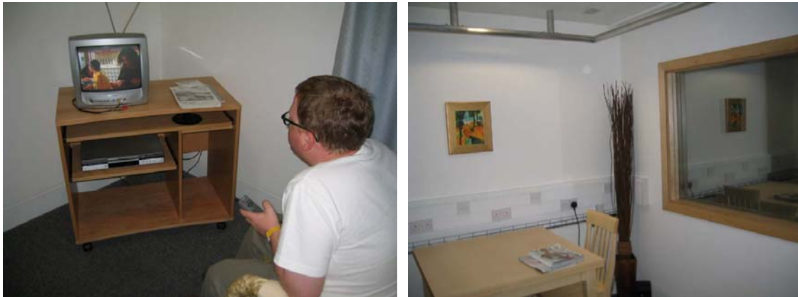
Figure 1. Usability lab with domestic furnishings: a) TV and DVD recorder on TV stand, with participant sitting in armchair to use remote controls; b) one-way glass window separating observation area (behind and to the left of the participant's armchair, from which this photograph is taken).
