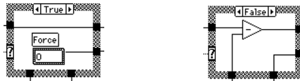
Figure 34 A LabView conditional from the rocket program, showing both arms. In the LabView environment, only one arm is visible on screen at any one time.
