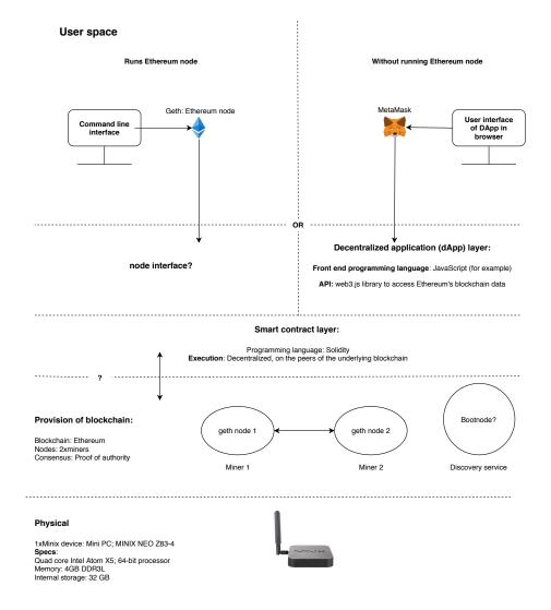
Figure 1: Overview of the experimental setup
