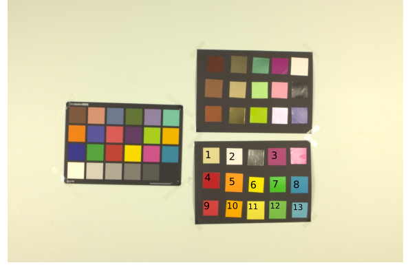
Figure 2: “Color Checker” on the left and “Color patches” on the right. Only the bottom target was used for testing as the top one contained non-diffuse materials with a complex BRDF. The HDR image was converted to the sRGB color space using the luminance of the white patch \times 1.5 as the peak luminance.
