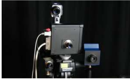
Figure 3.3: Cameras used in our experiment: HDRC VGAX (lower left), Silicon Vision Lars III (center), Jenoptik C14 (lower right), and Minolta LS-100 luminance meter (top).
