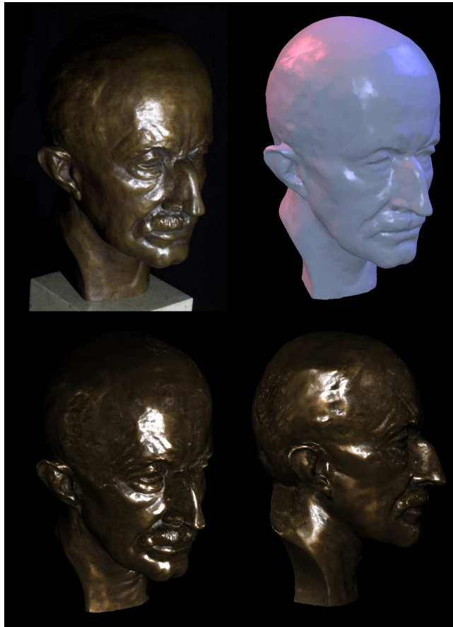
Figure 9.18: Digitalization of the Max Planck bust using the acquisition setup [154] shown in Figure 9.17: (upper left) photograph, (upper right) acquired 3D geometric model, (lower left) rendered image based on the acquired geometry model and spatially varying BRDF distribution for the same viewpoint as the photograph in (upper left), and (lower right) rendered image based on the same acquired model as in (lower right), but illuminated by different lighting and seen from a different viewpoint. Images courtesy of Hendrik P. A. Lensch, Jan Kautz, Michael Goesele, and Hans-Peter Seidel of MPI Informatik and Wolfgang Heidrich of the University of British Columbia.
