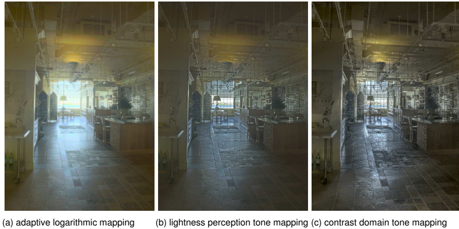
Figure 6.8: Different levels of detail visibility in tone mapping results. The increase in detail visibility is obtained at the cost of contrasts between larger image areas. The image (a) is the adaptive logarithmic mapping [64], (b) is the lightness perception tone mapping [14] and (c) is the contrast domain tone mapping [75]. Image courtesy of Byong Mok Oh.
