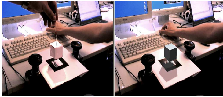
Figure 9.16: Real-world scene (left) and its augmented counterpart (right). The box floating over the table is a virtual object, which augments the video stream captured by the webcam (refer to Figure 9.15). The box is illuminated by lighting captured by the two HDR cameras. Images courtesy of Thorsten Grosch. Copyright the University of Koblenz-Landau.
