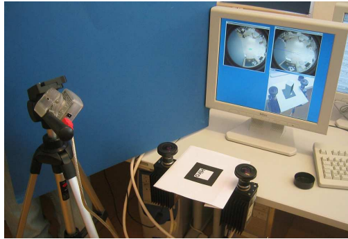
Figure 9.15: Light capturing system with stereo HDR video cameras (attached to the table). The webcam captures the scene view with the marker, which tracks position of the virtual object. The resulting augmented scene is shown on the display as well as two environment maps used to illuminate the scene. Image courtesy of Thorsten Grosch. Copyright the University of Koblenz-Landau.
