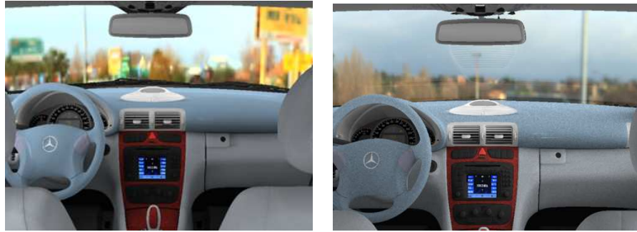
Figure 9.5: Snapshots of the car interior (left) rendered at interactive speeds using PRT techniques, and (right) computed off-line using the physically-accurate path tracing algorithm. Calibrated HDR VEMs have been used to model input lighting. Notice the cockpit reflections in the windshield for the path tracing image. Images courtesy of Tom Annen of MPI Informatik.
