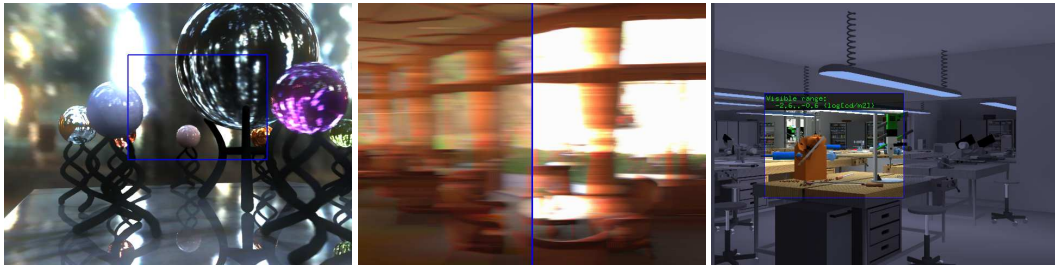
Figure 5.1: A range of perceptual effects that can be simulated based on HDR data. From left to right: visual glare (see light scattering at the edges of the objects); motion blur can be correctly simulated in linear luminance domain (right half); given absolute luminance values, color deficiency of night (scotopic) vision can be simulated. The source images courtesy of Paul Debevec, Spheron VR, and vr architects.
