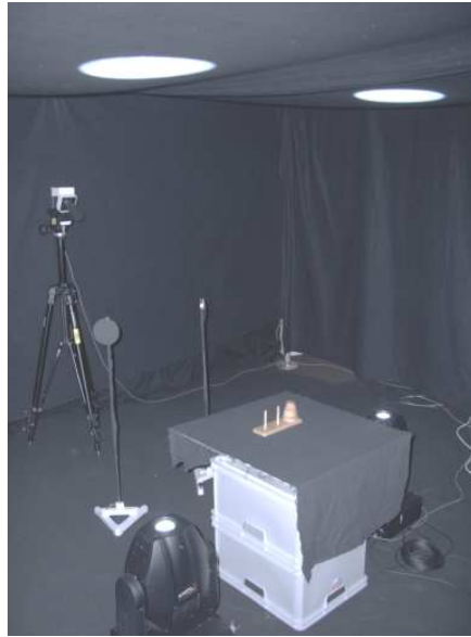
Figure 9.20: Photograph of a setup used for capturing of the 4D reflectance field [160]. Spotlight projectors placed on the floor illuminate a tent made of black cloth and indirectly illuminate the captured scene, which is arranged on top of the boxes. A camera mounted on the tripod records the HDR sequences with dynamically changing lighting due to computer controlled changes in the orientation of the spotlight projectors. Image courtesy of Martin Fuchs, Volker Blanz, Hendrik P. A. Lensch, and Hans-Peter Seidel of MPI Informatik.
