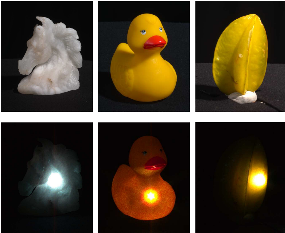
Figure 9.23: Translucent Objects Acquisition: (top row) the test objects used to capture their translucent appearance under indoor illumination and (bottom row) the same objects illuminated by a spot-shaped laser beam as captured by an HDR video camera using the acquisition setup shown in Figure 9.22 [161]. Images courtesy of Michael Goesele, Hendrik P. A. Lensch, Jochen Lang, Christian Fuchs, and Hans-Peter Seidel of MPI Informatik.
