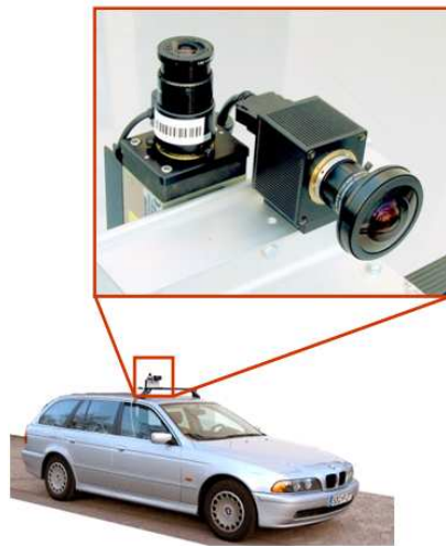
Figure 9.4: HDR video environment maps (VEM) acquisition system equipped with two photometrically-calibrated HDRC VGAx (IMS CHIPS) cameras for the sky lighting and windshield view capturing.
