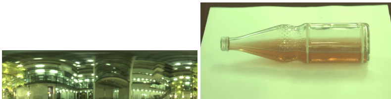
Figure 9.21: Rendering of the bottle containing a colored liquid (right) as re-lit by a real-world environment map (left) [160]. The image has been reconstructed using 1024 HDR images captured for different lighting conditions using the setup from Figure 9.20. Images courtesy of Martin Fuchs, Volker Blanz, Hendrik P. A. Lensch, and Hans-Peter Seidel of MPI Informatik.
