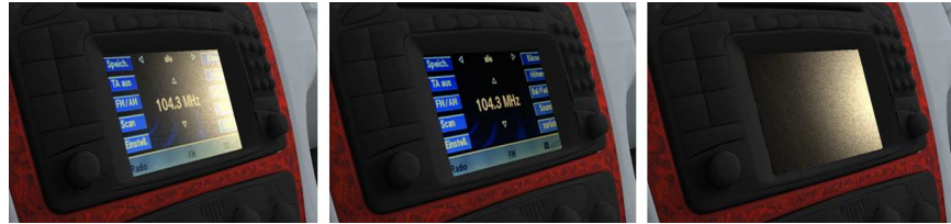
Figure 9.6: The LCD panel appearance as a result of the global illumination computation for VEM lighting: (left) full global illumination, (center) display emitted light only, and (right) reflected light. To compute the reflected light, BRDF-driven importance sampling and PRT lighting querying has been performed. Images courtesy of Tom Annen of MPI Informatik.
