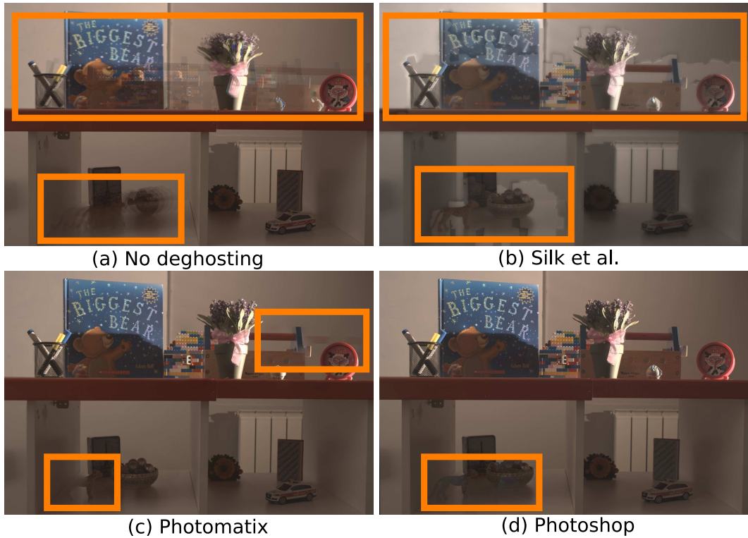
Figure 6: Tone mapped outputs of images generated by HDR deghosting algorithms, (image set 1, complex scene). Marked regions in images (a), (b), (c) and (d) show artefacts generated by No deghosting, Silk et al., Photomatix and Photoshop methods respectively. Images generated by Hu et al. and Sen et al. methods do not produce any visible ghosting artefacts and are therefore not shown in this figure.
