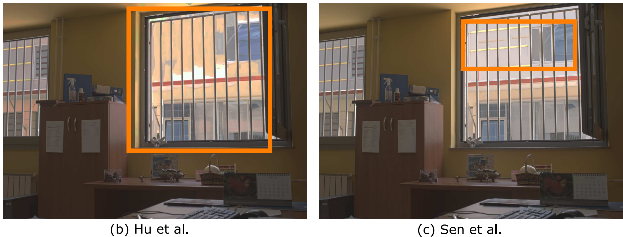
Figure 10: Outputs of images generated by (b) Hu et al.'s and (c) Sen et al.'s methods produce visible artefacts (image set 4, small object large motion scene). Marked region in image (b) shows reduced dynamic range produced by Hu et al.'s method in over-saturated region of the scene, and in image (c) ghost artefact produced by Sen et al.'s method.
