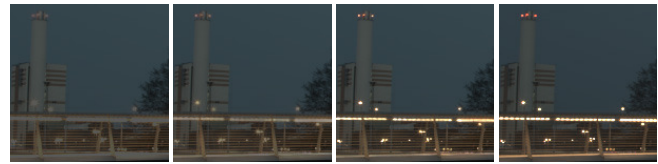
Fig. 8. A 150 \times 150 pixels zoom-in of a reconstruction. Using pre-training the CNN is in general more consistent and can reconstruct smaller highlights better.
