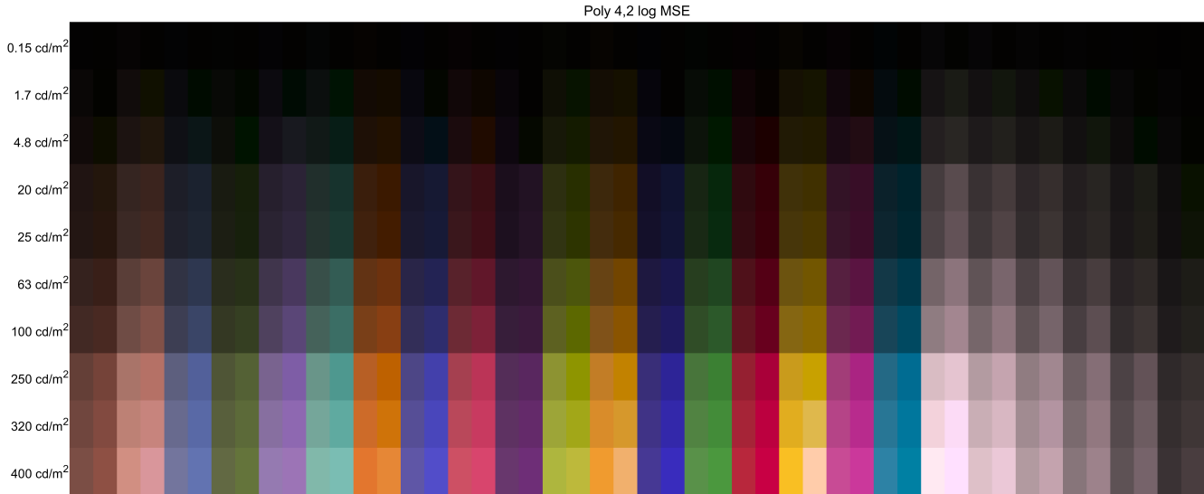
Figure 4. Approximate sRGB representation of the reference (left side in each patch) colors and the measured colors (right side in each patch) from the predicted RGB values from the 4th degree polynomial model ( r_{4,2} ) with E_{\log MSE} optimization loss function.
