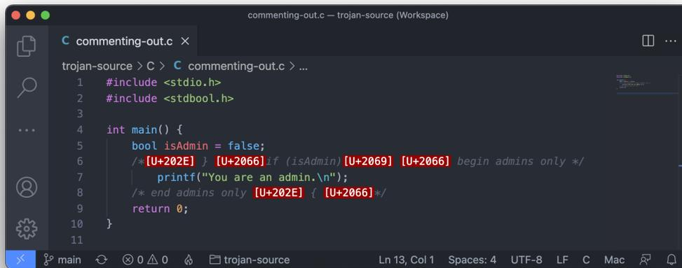
Figure 3.15: Trojan Source mitigations patched in Visual Studio Code
