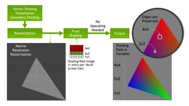
Figure 2.8: Variable rate shading allows visibility calculation at a full resolution and shading calculation at a lower resolution. Image from [Yang et al., 2019].
