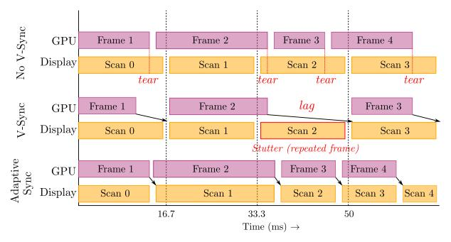
Figure 2.7: Display sync strategies. No synchronisation between rendering and display scan can lead to tearing artefacts. Synchronisation can introduce stuttering artefacts. Adaptive sync technologies eliminate both of these artefacts.
