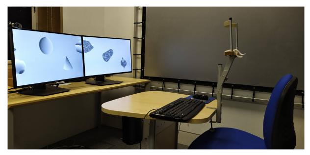
Figure 4.3: Experiment Setup. A chinrest was used to keep viewer's head at a fixed position.
