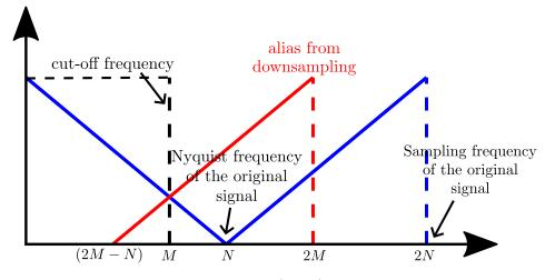
Figure A.2: Consider for example a 30 cpd (= N) signal displayed on a 40 ppd display. The maximum frequency the display can present (called the cut-off frequency) is 20 cpd (=M).
