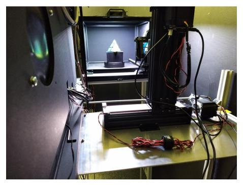
Figure 7.5: A gantry mounted with a DSLR camera is used to capture lightfield of the real scene
