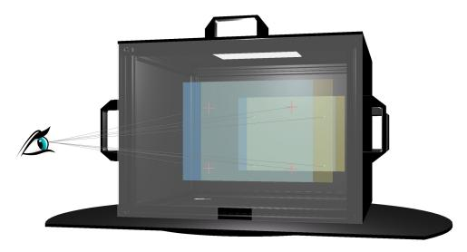
Figure 7.12: RSB with a detachable transparent plane with red markers. Users are asked to mark the pixels on all 4 displays (blue and yellow planes) corresponding to the 4 crosses and 4 LEDs on the back wall. This correspondence is used to calculate the transformation matrices for each display.
