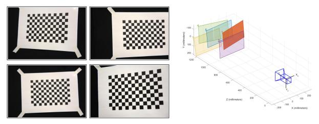
Figure 7.6: A printed checkerboard with known dimensions is used to calculate the camera's intrinsic matrix.
