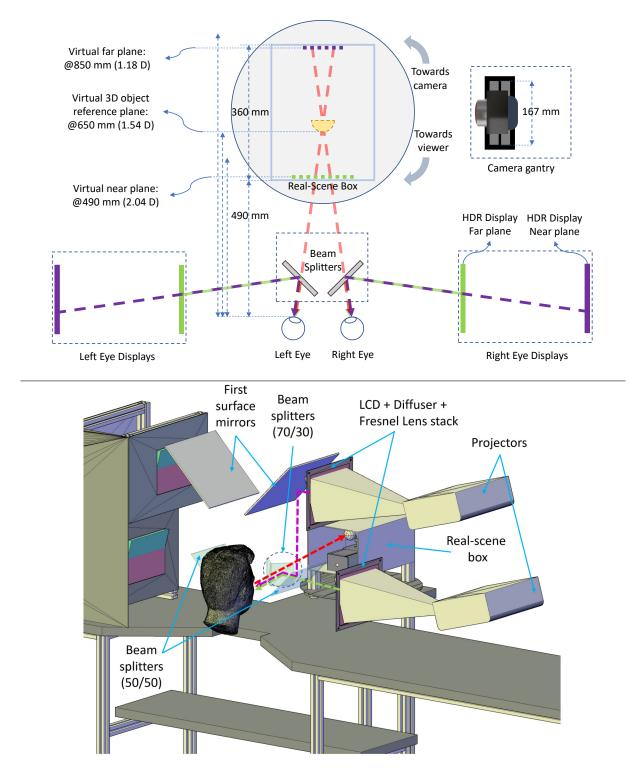
Figure 7.3: Schematic of the high-dynamic-range multi-focal stereo display apparatus. The beam splitters creates two virtual images per eye (green and blue dashed lines inside the real-scene box) overlapping with the physical scene in the real-scene box. The red, green, and purple lines depict the light paths from the displays and the physical scene to the eyes. The box can be rotated to face the camera gantry to facilitate the light field capture of the physical scene.
