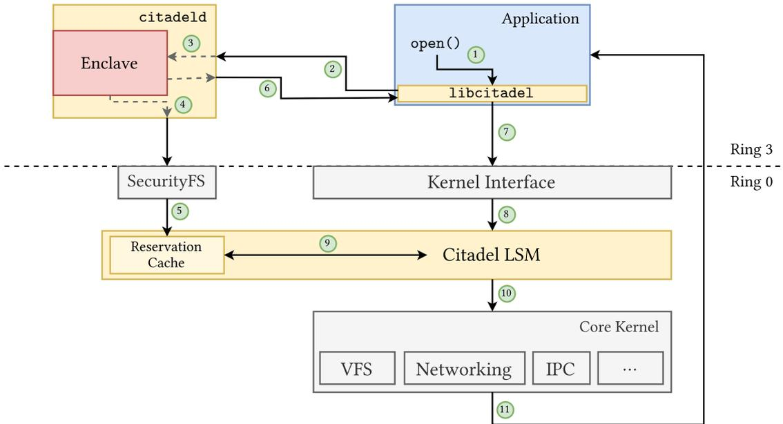
Figure 4.3: High level overview of the CITADEL architecture.
