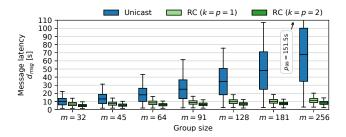
Figure 5: This box plot shows the distributions of message latency  $d_{msg}$  for increasing group sizes for the strategies *naïve* sequential unicast and Rollercoaster (RC). The Rollercoaster strategies show different k and p parameters. The boxes span from the first quartile to the third quartile (middle line is the median) and the whiskers indicate the 1st and 99th percentile.
