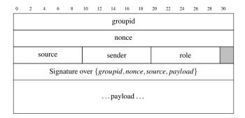
Figure 3: Payload header for the Rollercoaster scheme containing both the fields for the minimal scheme and the fields necessary for the fault-tolerance variant and further optimisations.
