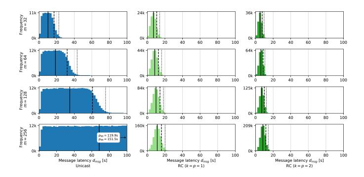
Figure 15: The distribution of message latency of naïve sequential unicast and Rollercoaster (RC) as perceived by the participating group members in a simulation where all users are online all the time. The solid line marks the mean latency whereas the dashed (and dotted) lines mark the  $p_{90}$  (and  $p_{99}$ ) latency. In this figure the y-axes are not linked in order to provide higher fidelity.
