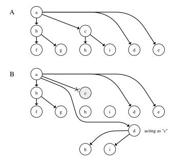
Figure 2: Message distribution graph for a group of size m = 9 and branching factor k = 2. Graph A: Expected delivery from source s = a. Graph B: The node c is offline and breaks delivery to h and i. Using the fault-tolerant variant the node d is assigned the role of c and delivers the payload to h and i.
