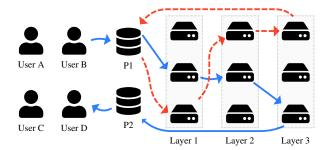
Figure 1: Schematic for a Loopix network with four users (A, B, C, D), two providers (P1, P2), and a three-layer mix network. Each node of mix layer L is connected to each node of layer L+1. The solid blue arrows depict one possible path for a payload or drop message from user B to user D. The dashed red line represents loop traffic induced by a mix node.
