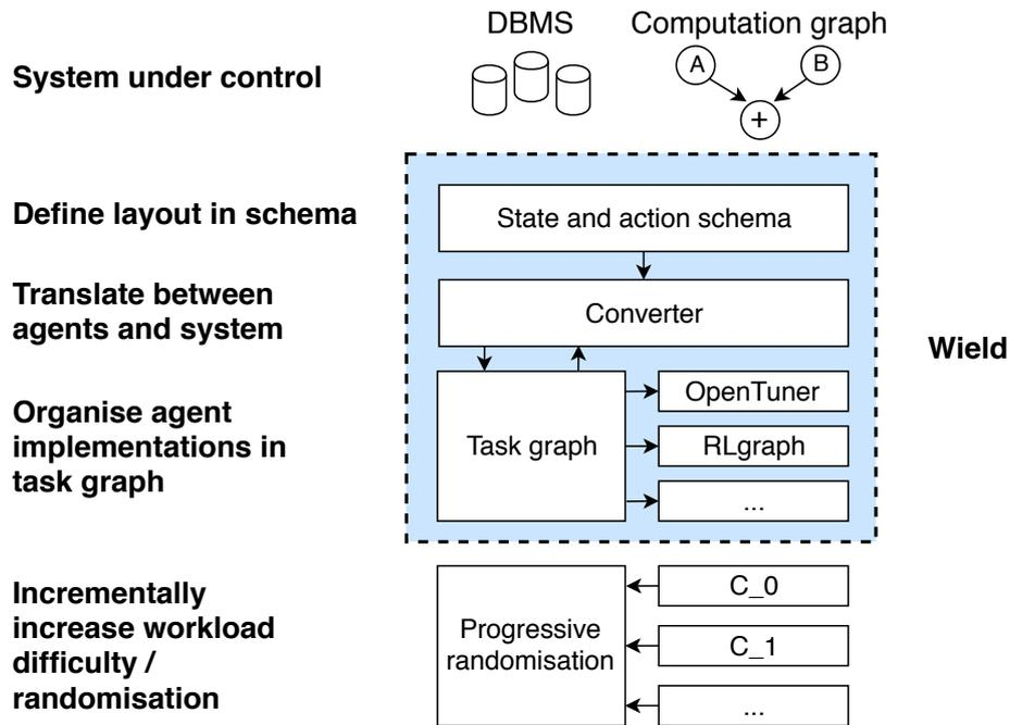
Figure 5.1: Conceptual overview of Wield in relation to existing auto-tuners, reinforcement learning frameworks like RLgraph, and systems.
