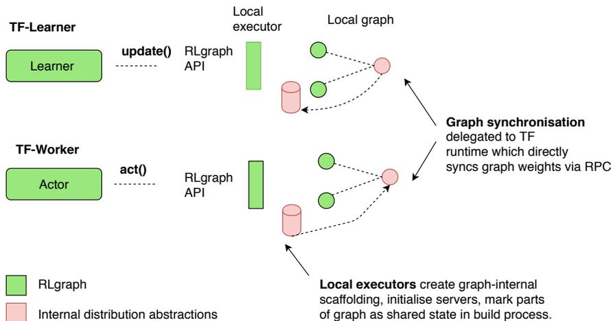
Figure 3.12: Graph-internal and graph-external distributed coordination.
