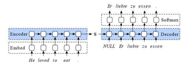
Figure 2.3: An overview of the encoder-decoder framework used in neural machine translation. An input sequence is encoded as a vector *s* which a decoder then translates based on this vector and all previously predicted words. The same principle applies to GEC.
