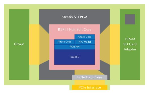
Figure 4.3: Block Diagram of the Attack Platform on the DE5-Net Board. 'Attack Code' is included twice, as different attacks can be carried out with and without the NIC model.
