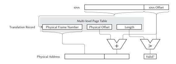
Figure 6.1: Diagram illustrating page table mapping with base and bounds. The use of the carry out bit as an additional validity check is not shown to simplify the diagram.
