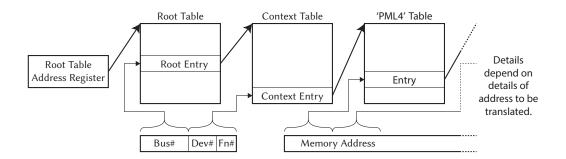
Figure 2.5: Diagram showing the page tables for Intel  $v\tau$ -d. The AMD table layout is similar, but the entirety of the PCIe requester ID indexes one much larger table – the first root table and context table are combined.
