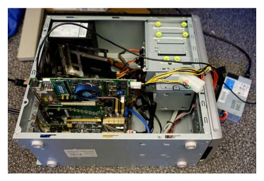
Figure 4.2: Photograph of Windows, Linux and FreeBSD experimental setup. This includes the FPCA in the riser for the PCIe analyser. The os was varied on the victim by replacing the hard drive.
