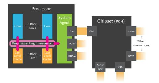
Figure 2.1: Diagram showing some of the different protocols that appear in a single-processor Intel system. If the system had multiple processors, these would be connected with Quick Path Interconnect. Intel's server class processors are beginning to move to a mesh-based internal interconnect, rather than the ring presented here [40].
