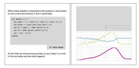
Figure 40: Function smoothing the X coordinate (left) with a sample run (right).
