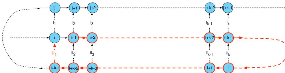
(c) Solving the constraint  $II_1$  in the Type II loop closure affects  $Pose_{i+1}$  to  $Pose_{i+k-1}$ .
