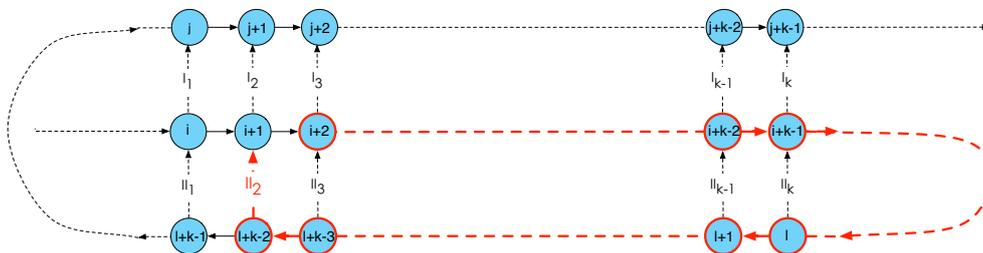
(d) Solving the constraint  $II_2$  in the Type II loop closure affects  $Pose_{i+2}$  to  $Pose_{i+k-2}$ .
