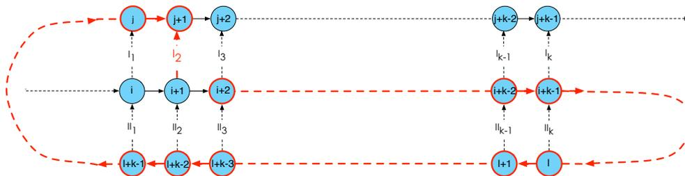
(b) Solving the constraint  $I_2$  in the Type I loop closure affects  $Pose_{i+2}$  to  $Pose_{j+1}$ .
