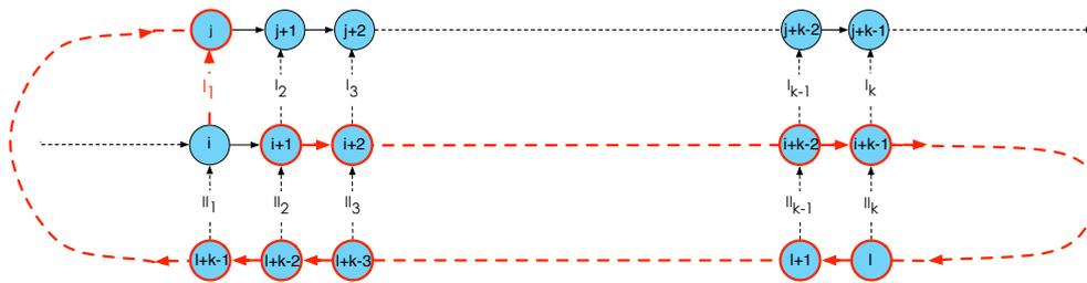
(a) Solving the constraint  $I_1$  in the Type I loop closure affects  $Pose_{i+1}$  to  $Pose_j$ .
