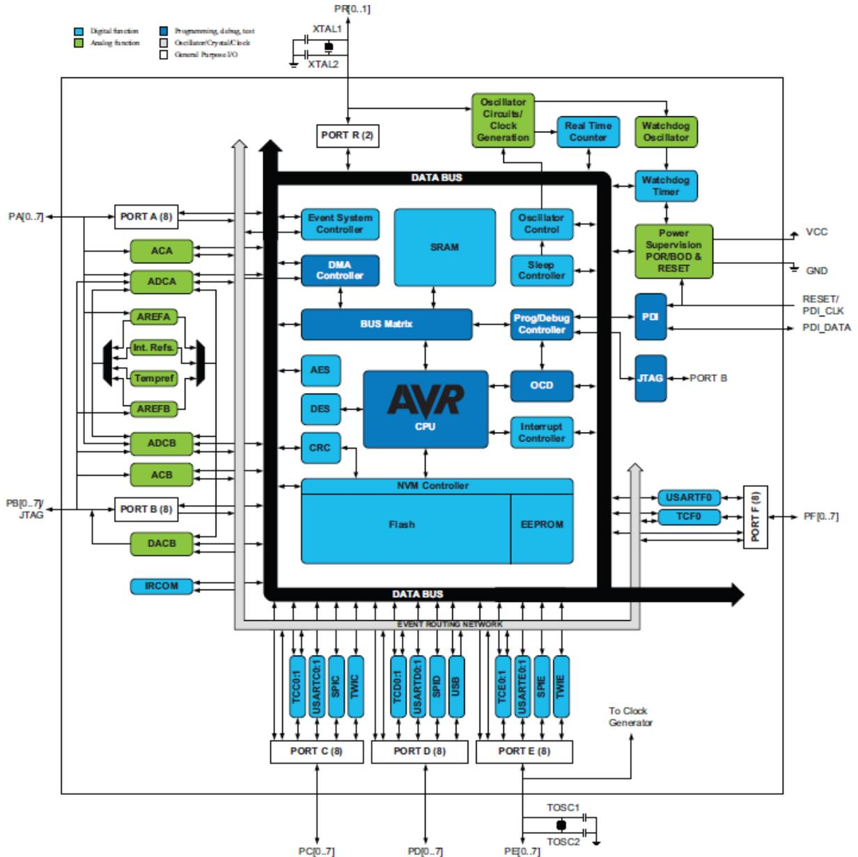
Figure 2.4: XMEGA A3U block diagram. Taken from the XMEGA A3U datasheet [31].
