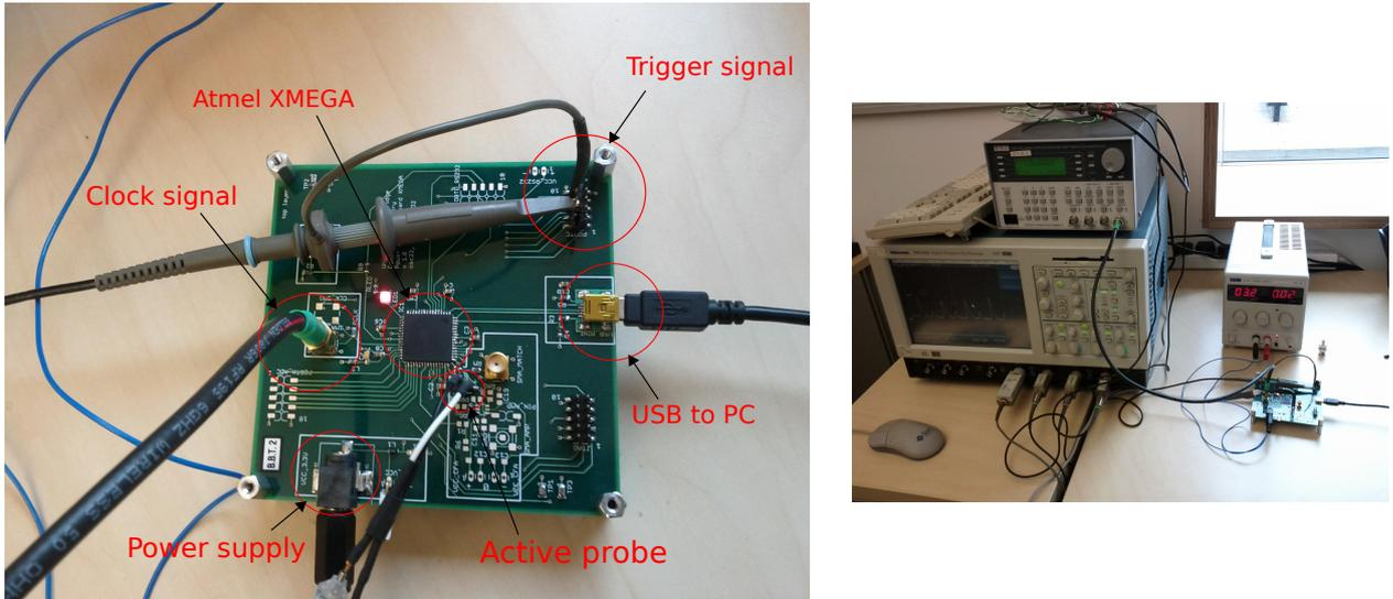
Figure 2.11: Left: XMEGA PCB while it was used for side-channel attacks. Right: overall acquisition setup.
