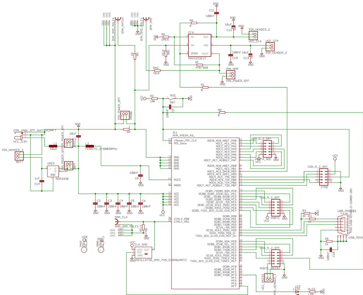
Figure 2.8: Schematic of the XMEGA PCB.
