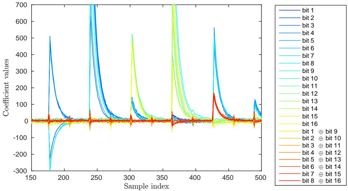
Figure 7.7: Contribution of coefficients  $\beta_{jb}$  in  $\mathcal{F}_{17}$  (bits 1 to 16) and  $\mathcal{F}_{17x}$  ( $\mathcal{F}_{17}$  enhanced with XOR between bits of 8-bit halves) for the *Panda* dataset. Pipelining causes leakage of the two 8-bit halves to overlap (e.g. around sample 300). Their consecutive processing also leaks their XOR value (e.g. around sample 430).
