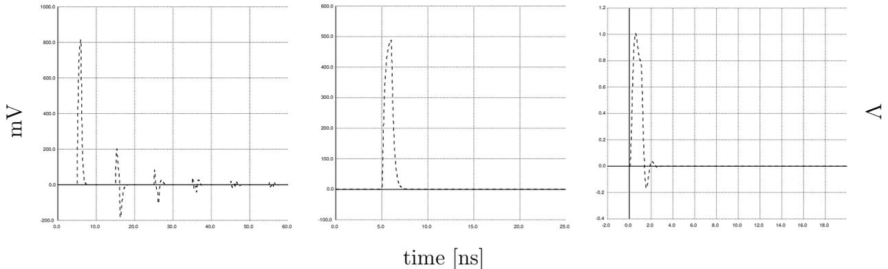
Figure 2.6: Voltage at the oscilloscope load from ngspice simulations. Left: standard circuit from Figure 2.5 (left), when  $I_S = 100$  mA. Centre: using a matching resistor at the source, as in Figure 2.7 (left). Right: using a *line does not matter* setup, as in Figure 2.7 (right).
