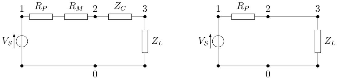
Figure 2.7: Thévenin equivalent circuit for *good* signal acquisition. Left: using matching resistor at the source. Right: ignoring  $Z_C$  when the line does not matter.
