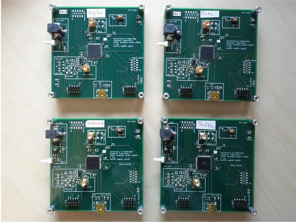
Figure 2.10: The four XMEGA PCB devices that I used in my experiments.
