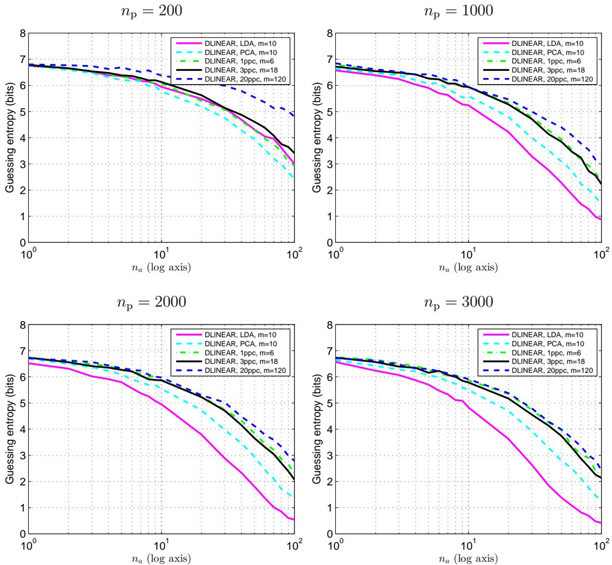
Figure 4.7: Guessing entropy after template attack on *Polar* dataset (AES engine), using different values of  $n_p$  and different compression methods.
