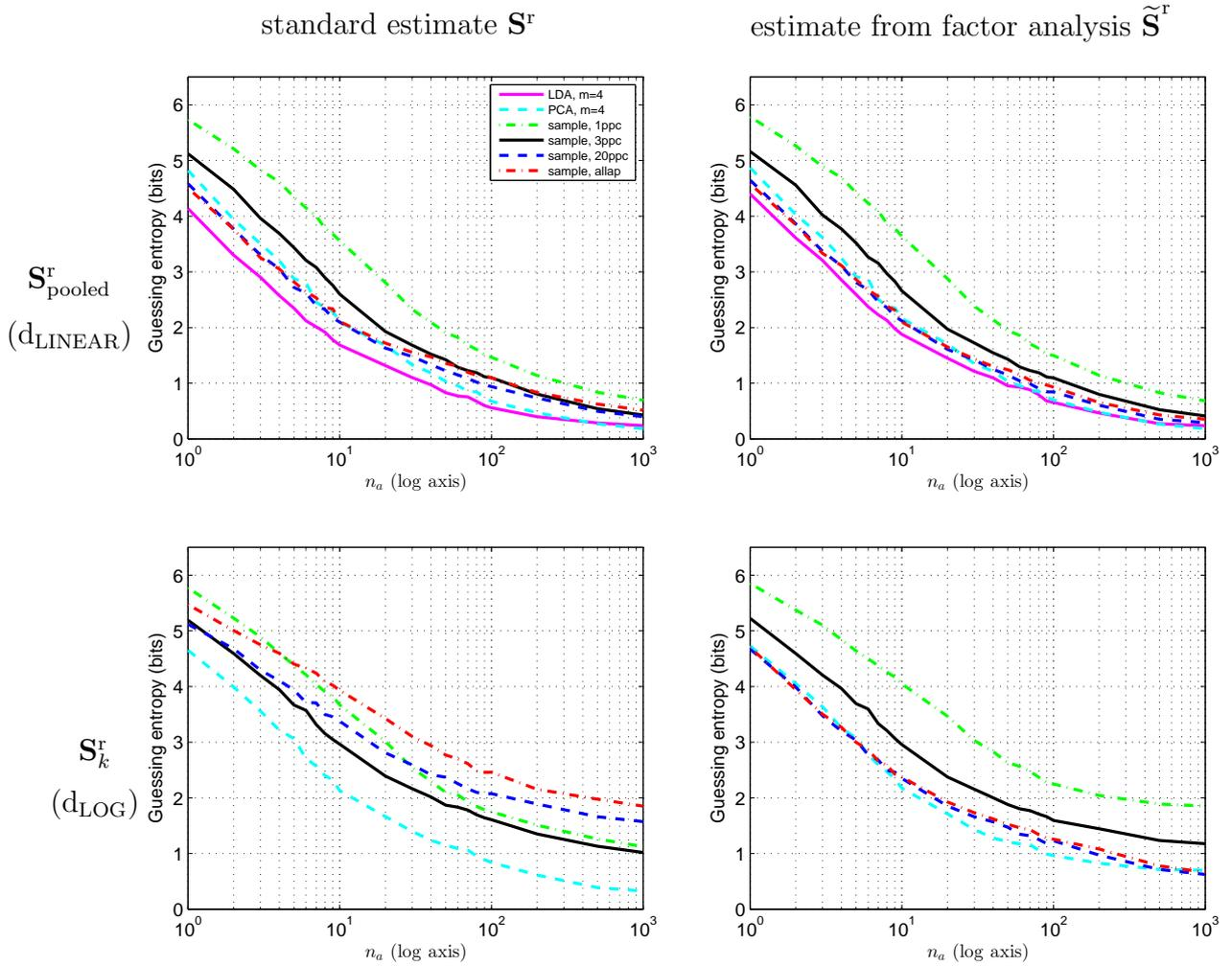
Figure 6.8: Results of template attacks on real data using the individual covariances with  $d_{\text{LOG}}$  (top) and the pooled covariances with  $d_{\text{LINEAR}}$  (bottom). Left: using the standard estimators for  $\mathbf{S}_k^r$  and  $\mathbf{S}_{\text{pooled}}^r$  from (4.1, 4.19). Right: using factor analysis to estimate  $\tilde{\mathbf{S}}_k^r$  and  $\tilde{\mathbf{S}}_{\text{pooled}}^r$ . In all cases I used  $n_p = 2000$  traces for each candidate  $k$  during profile.
