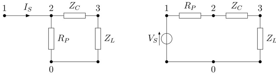
Figure 2.5: Circuit for signal acquisition (left) and Thévenin equivalent circuit (right).
