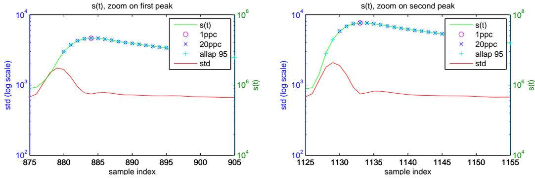
Figure 6.2: Signal strength estimate  $s_{\text{DOM}}$ , along with standard deviation for each sample points. Left: leakage samples around first clock cycle of target LOAD instruction; right: leakage samples around second clock cycle of the target LOAD instruction. Markers indicate the samples chosen using the sample-selection methods from Section 4.3.1.
