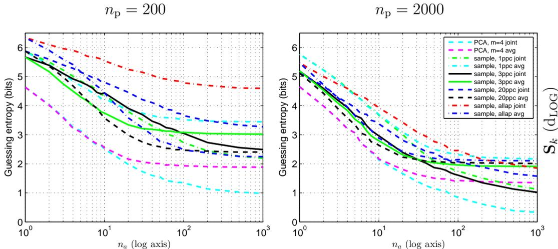
Figure 4.3: Guessing entropy remaining after template attacks, with different compressions, for  $n_p = 200$  (left) and  $n_p = 2000$  (right) profiling traces, using individual covariances  $\mathbf{S}_k$  with  $d_{\text{LOG}}$ .
