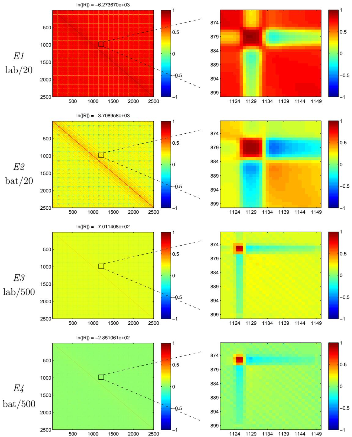
Figure 6.1: Sample correlation matrix  $\mathbf{R}$  for experiments  $E1$  to  $E4$ . Left: correlation between all sample points; right: correlation between samples around first and second peaks of signal strength estimate  $\mathbf{s}(t)$ .
