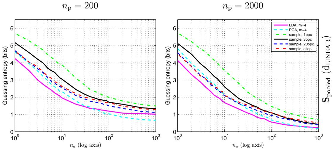
Figure 4.4: Guessing entropy remaining after template attacks, with different compressions, for  $n_p = 200$  (left) and  $n_p = 2000$  (right) profiling traces, using a pooled covariance  $\mathbf{S}_{\text{pooled}}$  with  $d_{\text{LINEAR}}$ .
