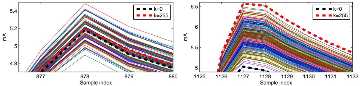
Figure 2.2: Average power consumption traces from the Atmel XMEGA A3U microcontroller, when loading different values from RAM memory to a register. Left: leakage at first clock cycle of LOAD instruction. Right: leakage at second clock cycle.
