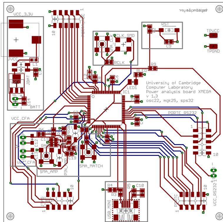
Figure 2.9: Board layout of the XMEGA PCB. Red: top side. Blue: bottom side.
