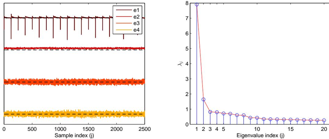
Figure 3.9: PCA eigenvectors (left) and eigenvalues (right) from leakage matrix  $\mathbf{X}_1$  ( $k = 1$ ) of *Grizzly Alpha* dataset.
