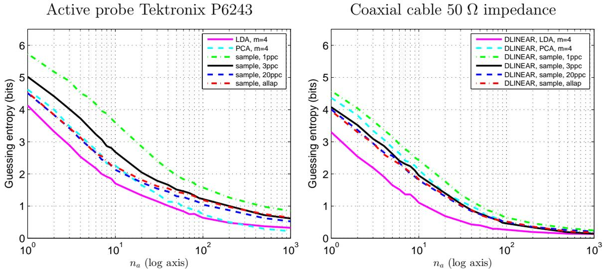
Figure 4.6: Guessing entropy after template attacks on the *Grizzly Beta* dataset, using the linear discriminant, and  $n_p = 1000$  profiling traces. Left: results using active probe Tektronix P6243; right: results from using a coaxial cable with  $50\ \Omega$  characteristic impedance, connected to the matched line of the XMEGA PCB.
