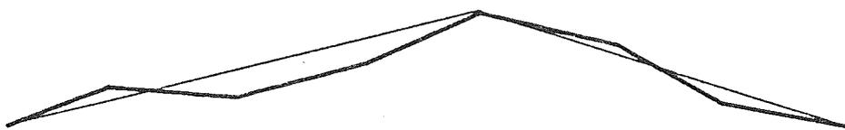
The furthest points in both sections are now less than the tolerance and so these sections can be replaced by straight lines.
