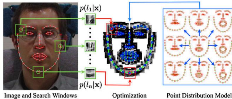
Figure 4.2: Two step CLM fitting: calculation of patch responses in the surrounding region of interest followed by a Point Distribution Model constrained parameter update. Taken from [Saragih et al. \(2011\)](#).
