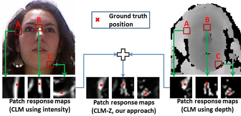
Figure 5.2: Response maps of three patch experts: (A) face outline, (B) nose ridge and (C) part of the chin. SVR patch expert response maps using greyscale intensity contain strong responses along the edges, making it hard to find the actual feature position. By integrating response maps from both intensity and depth images, the CLM-Z approach mitigates the aperture problem.
