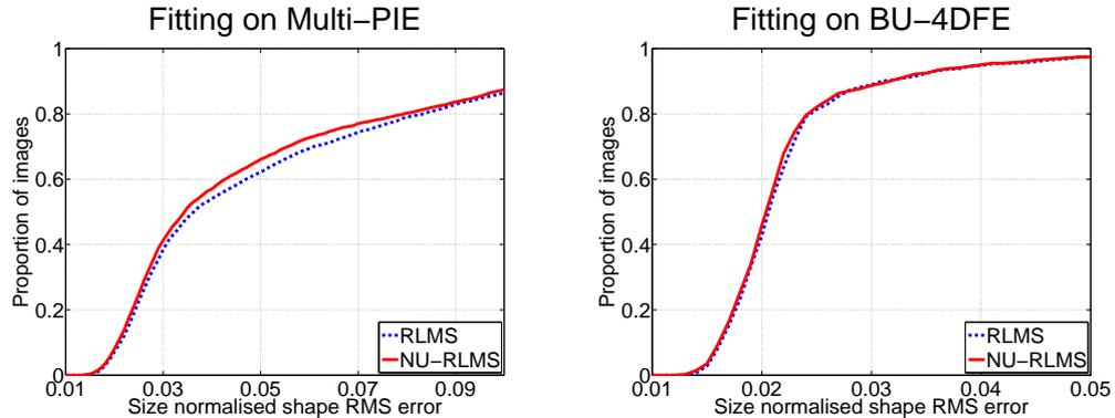
Figure 4.17: Error fitting curves when using RLMS and NU-RLMS algorithms. NU-RLMS increases landmark detection accuracy on both of the datasets, although the increased accuracy is marginal on the BU-4DFE dataset.
