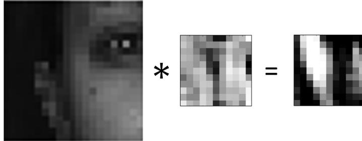
Figure 4.7: Example of a  $11 \times 11$  pixel area of interest ( $21 \times 21$  pixel grid) being convolved with  $11 \times 11$  pixel SVR patch expert weights, resulting in a  $11 \times 11$  pixel response. This response can be used to calculate the final response map using logistic regression. The darker response values indicate low probability of alignment, and brighter values indicate high probability of alignment.
