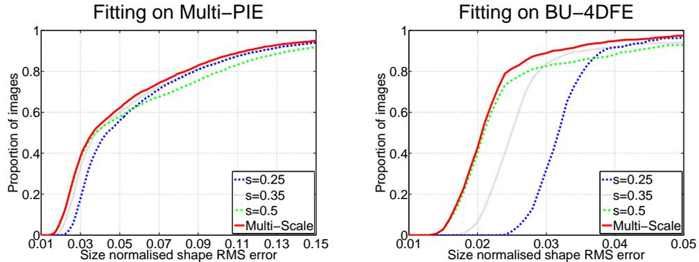
Figure 4.18: Error fitting curves when using different scale patch experts for CLM fitting. Notice how the robustness degrades as the scaling term grows larger (more images with high error), but the accuracy improves (more images with low error) leading to a trade-off. Multi-scale formulation, however, manages to retain both robustness and accuracy leading to better performance.
