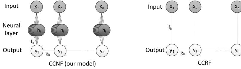
Figure 8.1: The linear-chain CCNF model compared to the linear-chain CCRF one (Section 7.3). The input vector  $\mathbf{x}_i$  is connected to the relevant output scalar  $y_i$  through the vertex features that combine the  $h_i$  neural layers (gate functions) and the vertex weights  $\alpha$ . The outputs are further connected with edge features  $g_k$
