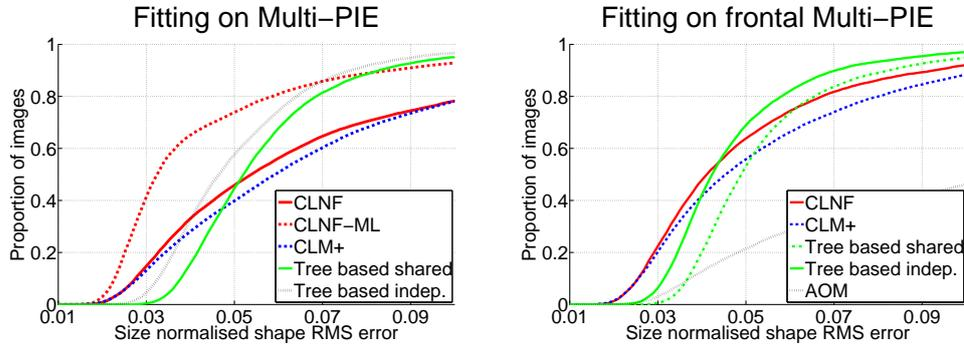
Figure 6.10: Comparison of CLNF and other landmark detectors on the Multi-PIE dataset, but on unseen to training illumination (except for CLNF-ML case which is there only for reference). Notice how the performance drops on unseen illumination, however the drop for a holistic approach (AOM) is the greatest.
