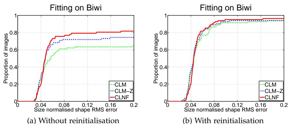
Figure 6.12: Error fitting curves on the Biwi Kinect head pose dataset using the CLNF approach versus CLM and CLM-Z. Normalised by interocular distance.
