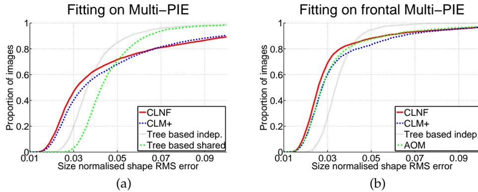
Figure 6.9: Comparison of CLNF and other landmark detectors on the frontally lit Multi-PIE dataset. a) The performance on the whole dataset. b) The performance on the close to frontal images (from  $-15^\circ$  to  $15^\circ$  yaw). Notice how CLNF outperforms all of the other approaches in terms of accuracy, but the tree based models of [Zhu and Ramanan \(2012\)](#) are better in terms of robustness.
