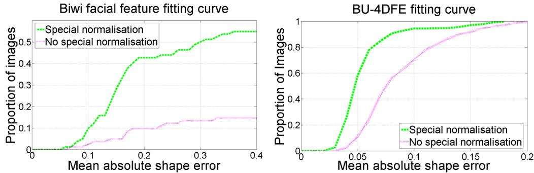
Figure 5.4: The fitting curve of CLM-Z comparing how the use of the specialised depth normalisation affects the landmark tracking accuracy. Note the much higher fitting accuracy on depth images using the normalisation scheme  $\mathcal{P}_Z$ , as opposed to zero mean unit variance one. This is especially evident on Biwi dataset which has a much noisier signal due to Kinect sensor.
