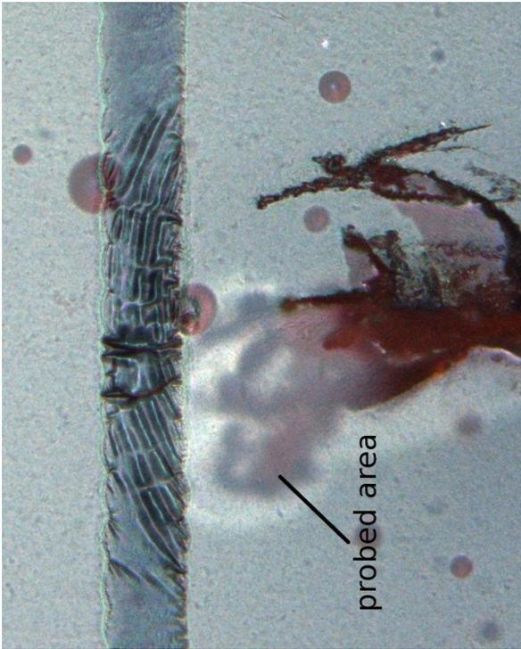
(a) Probe needle pushed next to PEDOT line
