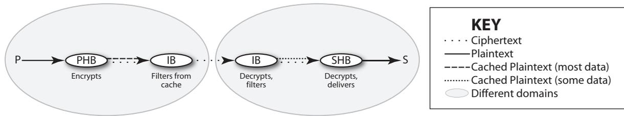
**Figure 7.2:** Caching decrypted data can increase efficiency when delivering an event to a peer with similar privileges.
