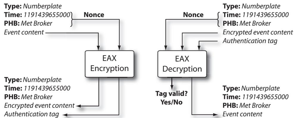
**Figure 7.4:** The EAX mode of operation.
