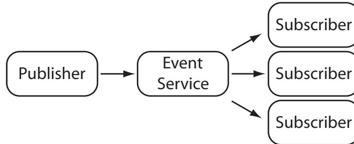
**Figure 2.1:** The event service and the use of asynchronous messaging decouples the publisher from the subscribers in time, space, and synchronisation.
