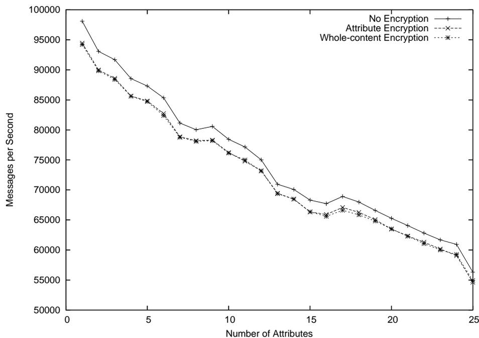
**Figure 7.9:** The end-to-end throughput of events with plaintext events, event level encryption, and attribute level encryption when plaintext caching is enabled.
