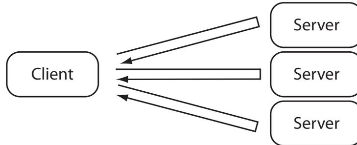
**Figure 2.2:** The use of synchronous messaging and the lack of an intermediary couples the client tightly to the server.
