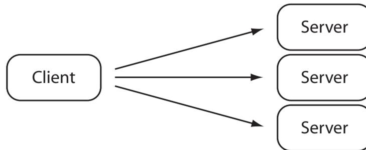
**Figure 2.3:** In traditional message passing the use of asynchronous messaging achieves synchronisation decoupling between the message producer and the message consumer.
