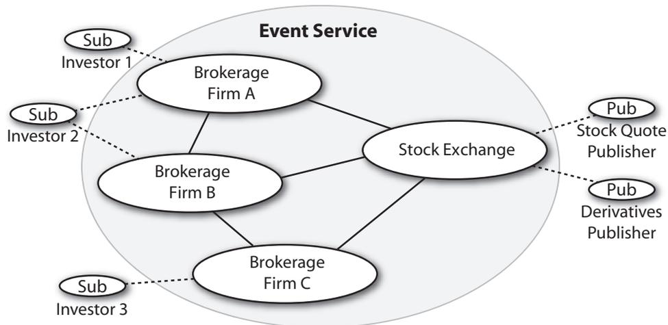
**Figure 1.3:** A multi-domain publish/subscribe system consisting of three brokerage firms and one stock exchange.
