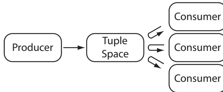
**Figure 2.6:** The *rd* operation in a Tuple Space allows many-to-many interaction between producers and consumers.
