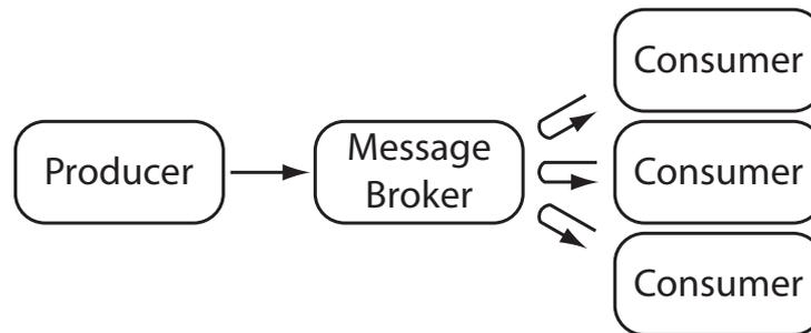
**Figure 2.4:** In a message queueing system the message broker decouples the producer from the consumers in time and space, but the consumers need to pull messages from the broker synchronously.
