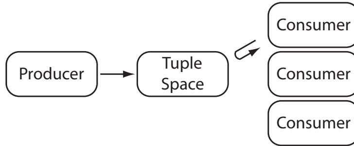
**Figure 2.5:** The *in* operation supports a many-to-one interaction model.
