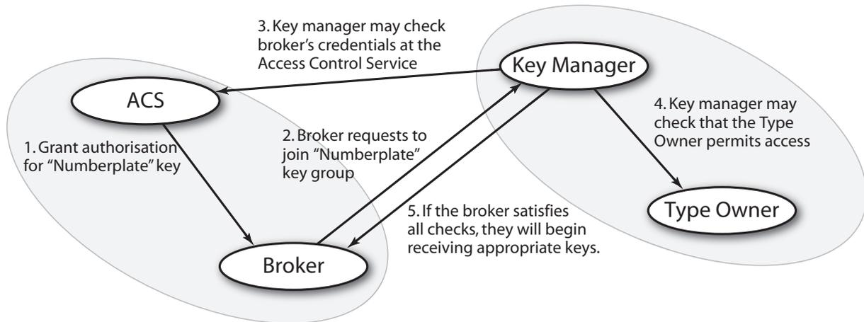
**Figure 7.5:** The steps involved for a broker to be successful in joining a key group.
