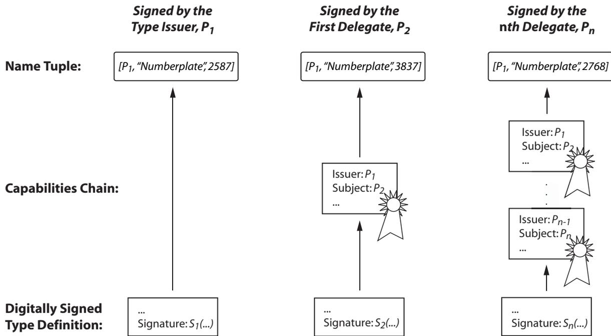
**Figure 4.4:** Verifying the name-signature link with and without a capabilities chain.
