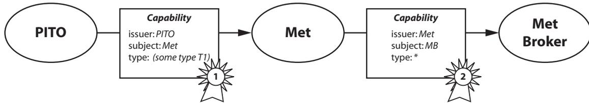
**Figure 5.2:** The blanket capability together with the capability issued to the Met domain authorises the broker to access type  $T_1$ .
