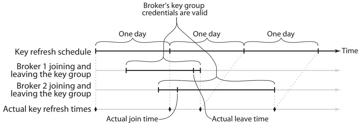
**Figure 7.6:** Key refreshes can be delayed based on the validity times of the broker's authority.
