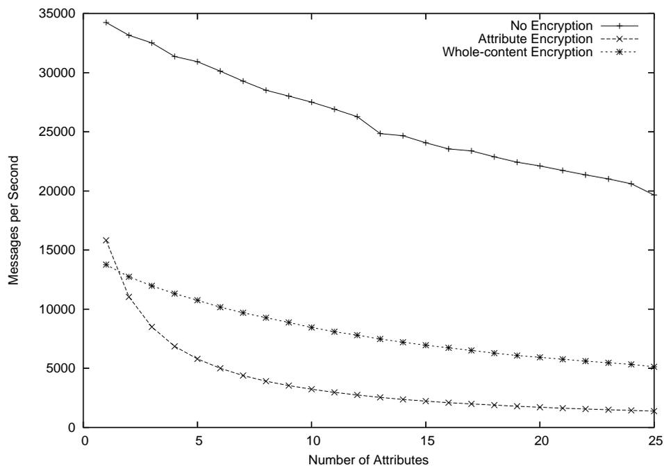
**Figure 7.8:** The end-to-end throughput of events with plaintext events, event level encryption, and attribute level encryption.
