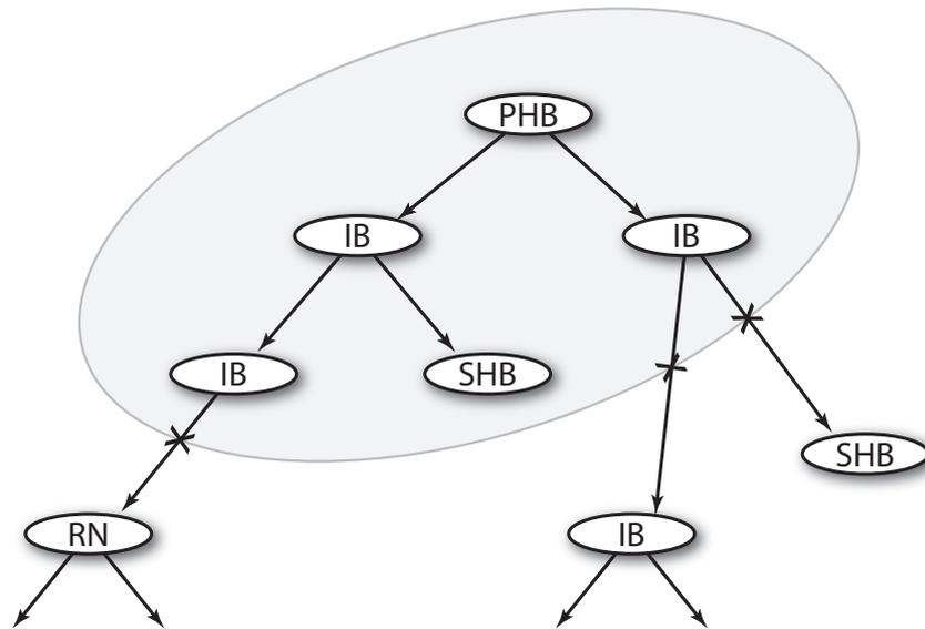
**Figure 7.3:** Node addressing is effectively random, therefore the rendezvous node for a domain internal type can be outside of the domain that owns an event type.
