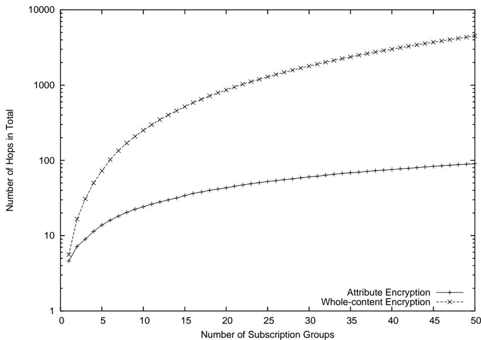
**Figure 7.10:** The average number of hop counts when emulating attribute level encryption with event level encryption and multiple sub-types (log scale).
