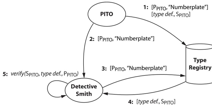
**Figure 4.1:** Detective Smith retrieves the Numberplate event type definition from a type registry and verifies its authenticity and integrity.
