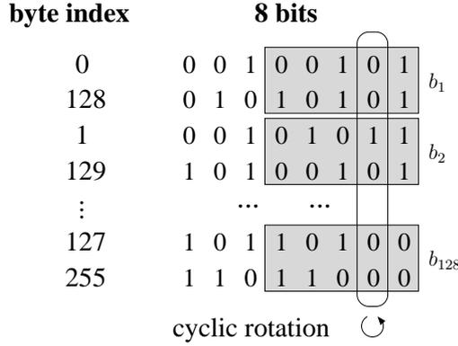
Figure 4.5: Permutation by rotating bit columns
