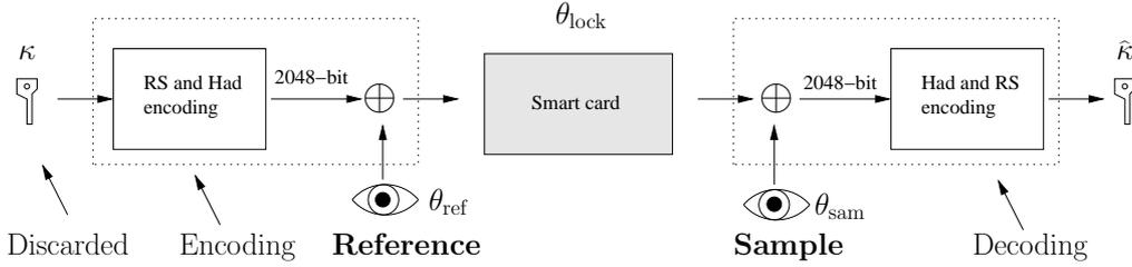
Figure 3.1: A two-factor scheme for biometric key generation
