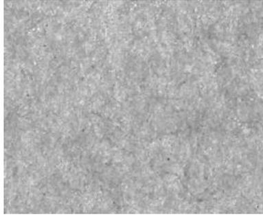
Figure 2.1: Translucency patterns over  $1 \text{ mm}^2$  of a sheet of paper
