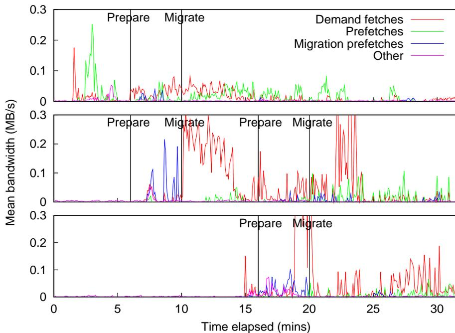
Figure 6.13: The bandwidth profile at 5 second sample intervals across three nodes as a virtual disk is migrated across them. Each graph's Y axis ranges from 0 to 0.3MB/s. The vertical red lines indicate, as labelled, the times at which migration was notified to the source node, and at which migration was then enacted.
