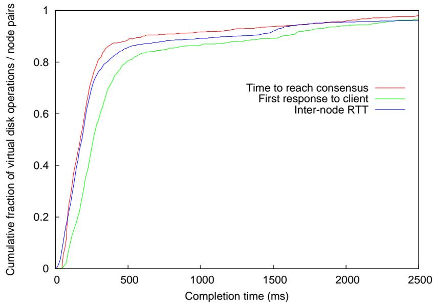
Figure 6.12: The cumulative distribution of completion time of virtual disk operations. The series show both the time to achieve consensus between managers and the client-perceived latency.
