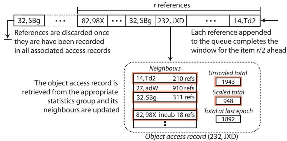
Figure 4.2: Updating an object access record
