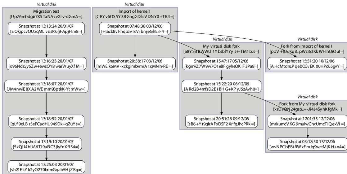
Figure 3.10: The assignment of volumes to virtual disks. A *Xest* utility generated this figure using the GraphViz package. The first fork from each snapshot volume may be appended inside the same virtual disk. Subsequent forks must instantiate a new virtual disk.
