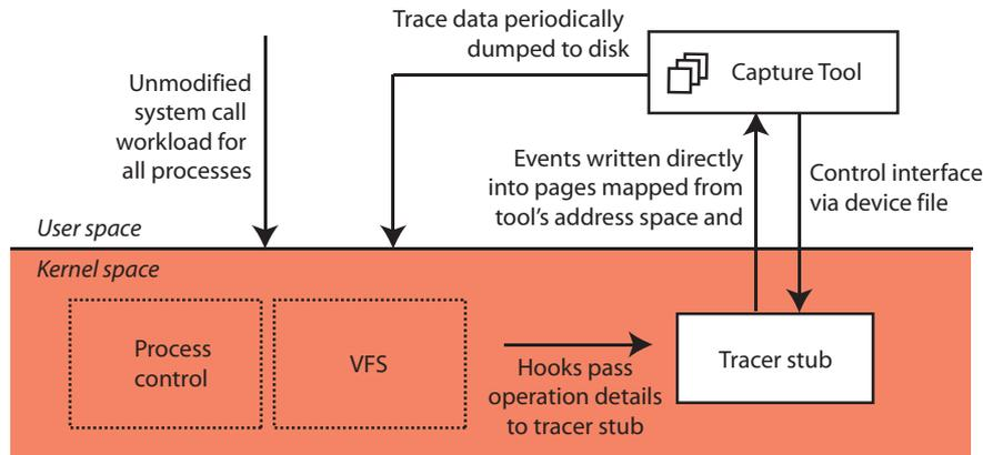
Figure 5.2: The structure of the VFS trace toolkit
