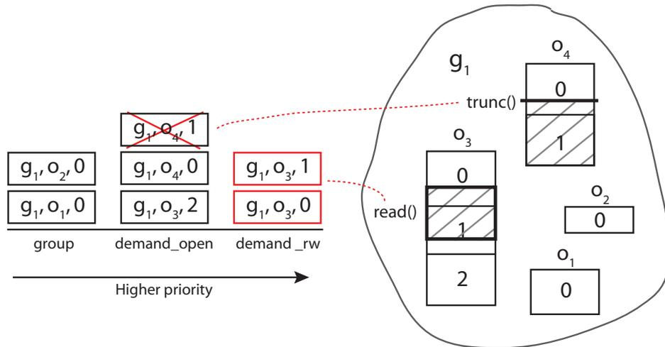
Figure 3.8: An illustration of fetch prioritisation. Objects  $o_3$  and  $o_4$  have been opened, causing their chunks to be fetched at priority `demand_open` and the chunks of other objects in the group at priority `group`. Next, a read on  $o_3$  elevates the priority of the covered chunks to `demand_rw`. Finally, a truncate on  $o_4$  causes ones of its fetches to be cancelled.
