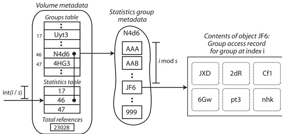
Figure 4.1: Storage of a volume's statistics. The volume metadata's statistics table is used to identify statistics groups, whose objects each contain a single group access record. The figure illustrates how the group access record is located for groups table index  $i$ . The constant  $s$  denotes the maximum number of regular groups on which a statistics group holds details.
