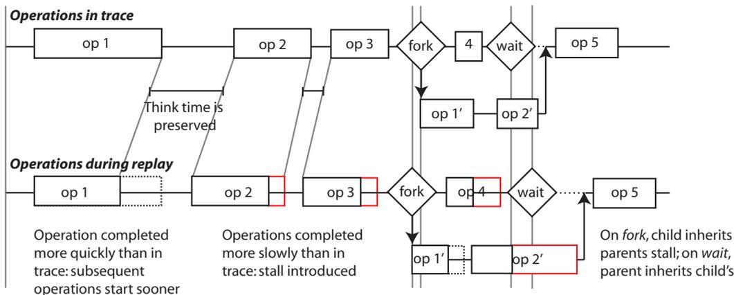
Figure 5.4: Dependencies between traced operations.
