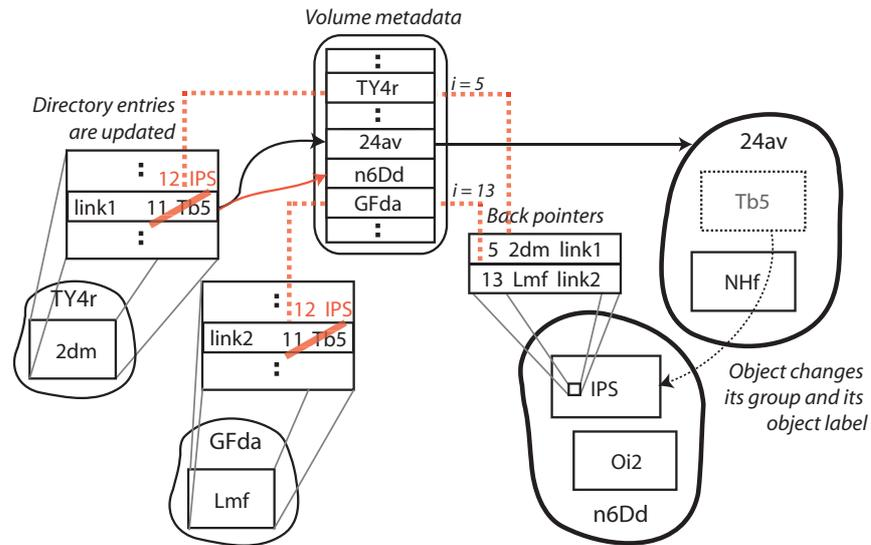
(a) Repairing directory entries using a relocated object's back pointers
