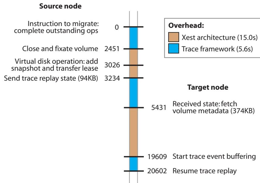
Figure 6.14: The steps taken in migrating access to a volume. Times given are in milliseconds and refer to the recorded times from the first transfer shown in Figure 6.13.
