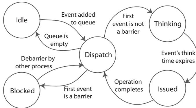
Figure 5.5: State transition diagram for simulating traced processes.
