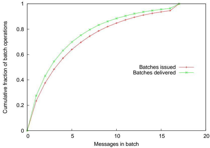
(a) The cumulative distribution of the number of pointer insertion requests in a batch, across all nodes, on forwarding from the batch's source node and on delivery to its destination.
