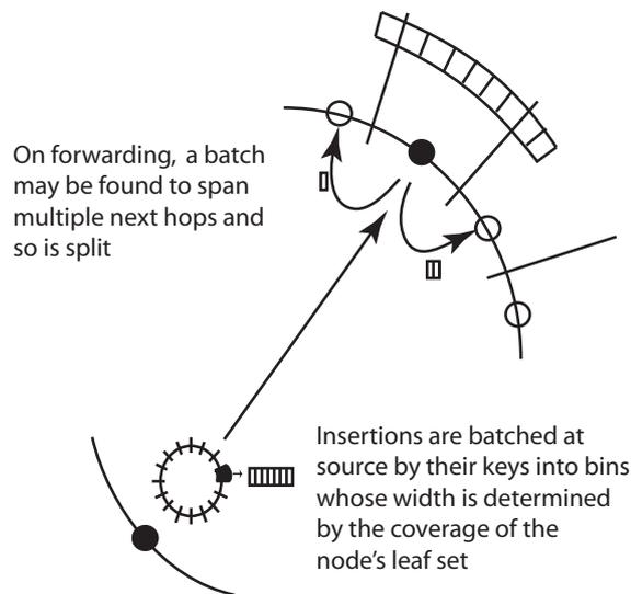
Figure 3.7: Routing batched requests through the DHT.
