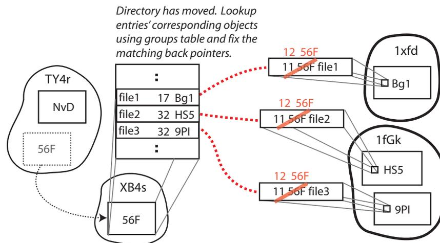
(b) Repairing back pointers using a relocated directory's entries. Objects are located, as usual, using the volume metadata's groups table, not shown in this figure.
