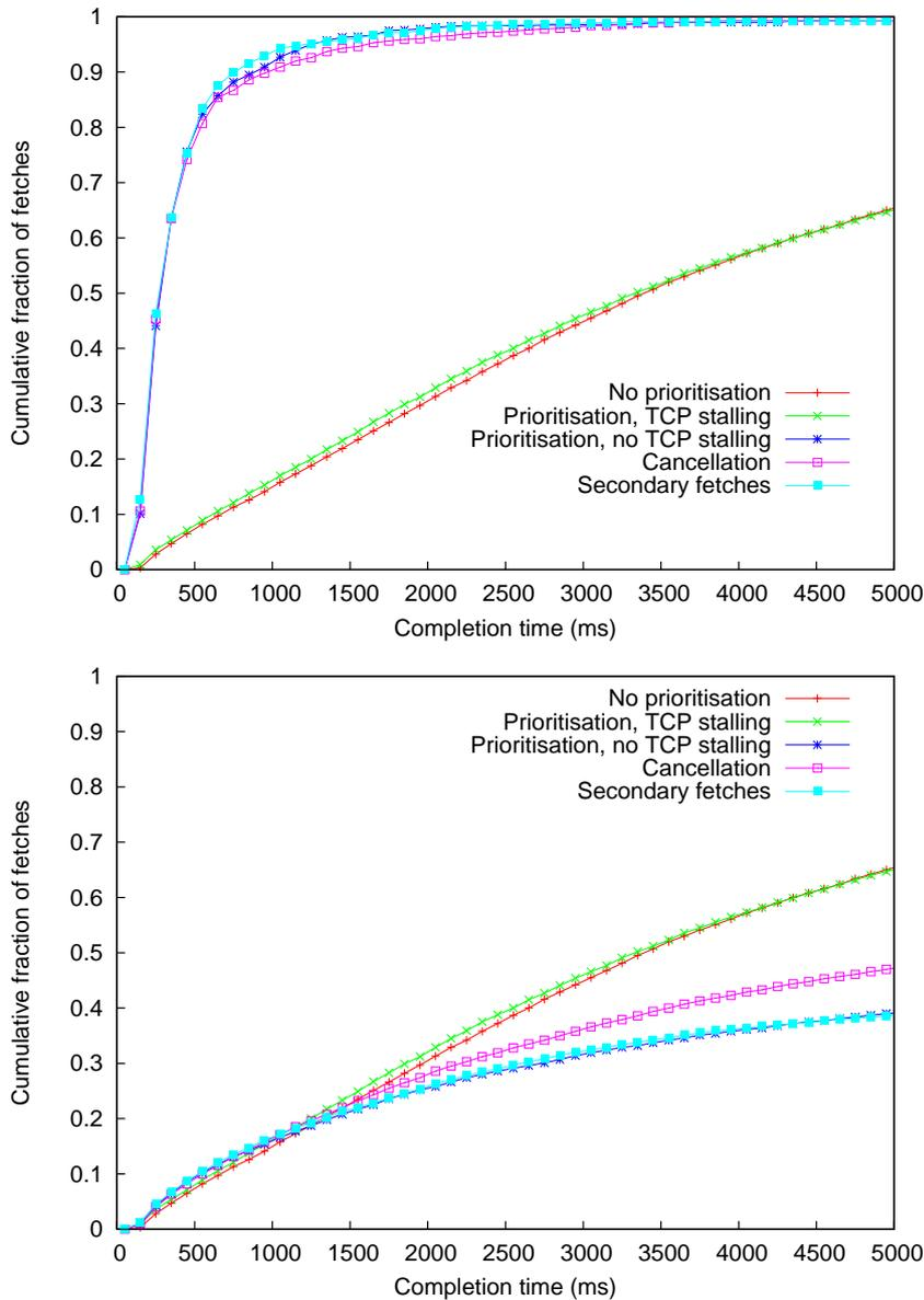
Figure 6.11: The effect of fetch protocol optimisations on the completion time of: (a) objects whose priority at the point of completion was demand; and (b) all object retrieval operations.
