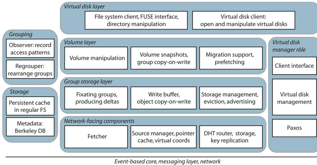
Figure 3.1: The structure of the *Xest* prototype.
