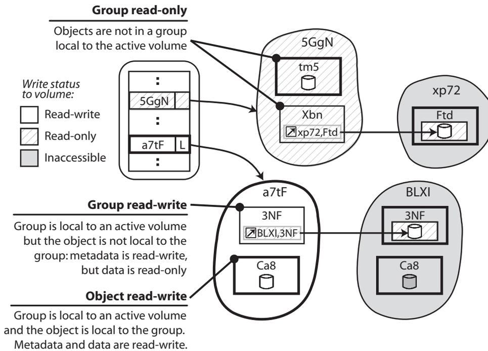
Figure 3.4: Determining the write status of an object for an active volume. An object local to its group has an emphasised border; a group local to the volume likewise. Cylinder symbols indicate the presence of associated object data. Objects (a7tF,3NF) and (5GgN,Xbn) are both pointers, and only their targets' data, not its metadata, is accessible. Observe that the metadata of (a7tF,3NF) is read-write because group a7tF is local to the volume, as marked in its group table entry.
