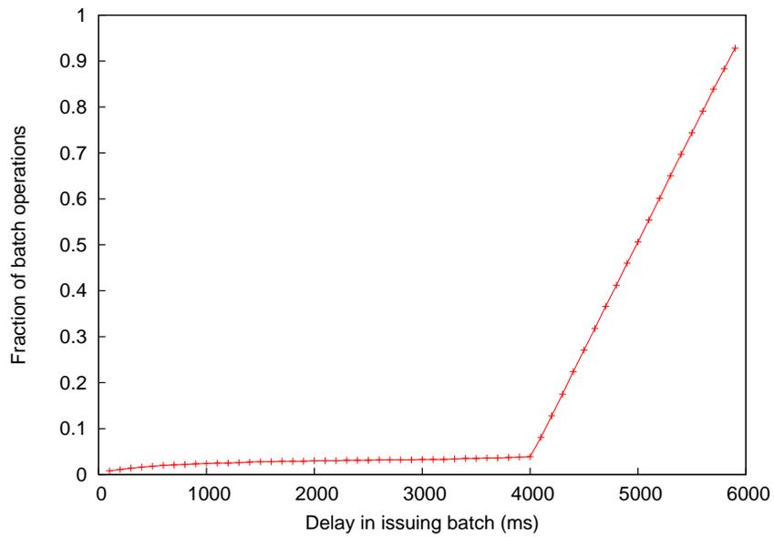
(b) The distribution of the delay with which a batch is issued after its first constituent request is made. The peak at 6 seconds is explained in the text.
