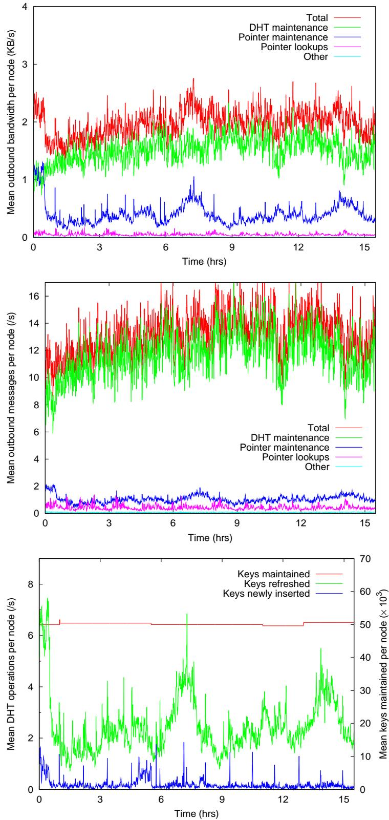
Figure 6.9: The cost of maintaining the DHT and its contents for each node in terms of: (a) out-bound bandwidth; (b) messages sent; (c) DHT storage operations.
