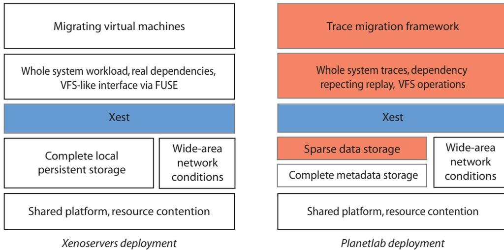
Figure 5.1: Approximating a Xenoserver deployment over PlanetLab. Due to feature and resource constraints imposed by the PlanetLab environment, the workload of a set of migrating virtual machines must be simulated, and storage of data conducted sparsely.
