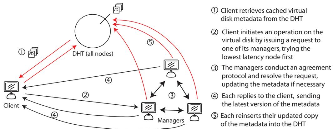
Figure 3.11: Operations on virtual disks.
