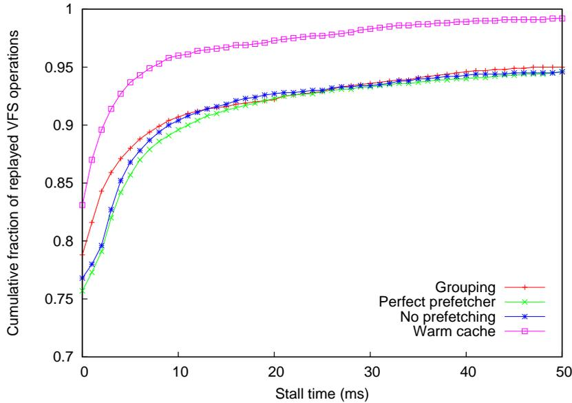
Figure 6.6: Cumulative distribution of the stall time of replayed VFS operations during virtual machine startup. Stall times are measured with respect to the time taken for the same operation as recorded in the trace, not to warm cache conditions. Note the range of the axes.
