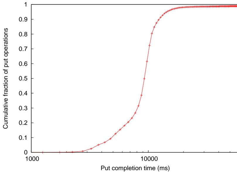
Figure 6.8: The cumulative distribution of completion times of pointers insertions. Note the logarithmic scale. Batching occurs before the insertion is routed through the DHT, before it is forwarded to each member of the destination node’s leaf set, and before a reply is returned to the client.
