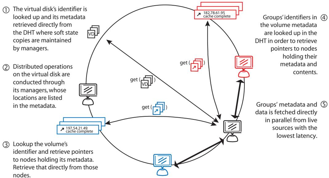
Figure 3.6: The rôle of the DHT in accessing file system data. The client, bottom right, first retrieves the virtual disk's metadata, then locates its managers, and looks up and fetches volume and group metadata.
