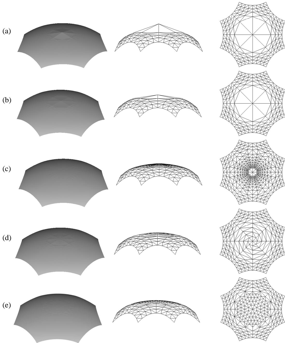
Figure 1: Bounded curvature Catmull-Clark [Augsdörfer et al., 2006] applied to an elliptic shape with an extraordinary vertex of valency eight at its centre. In each case the rendered surface is shown on left, and the polygon edges in the centre and at right. (a) basic subdivision, (b) vertices pushed to the limit surface, (c) adaptive subdivision, (d) Bézier curves on spoke edges, (e) Bézier patches between spoke edges.
