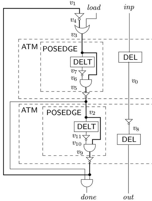
Figure 4.1: Combinational loop in  $(\text{SEQ} (\text{ATM} (\lambda x. x)) (\text{ATM} (\lambda x. \neg x)))$ .
