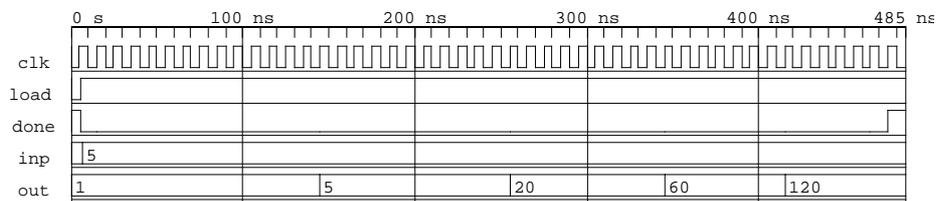
Figure 4.5: Well-behaved simulation of factorial of 5.
