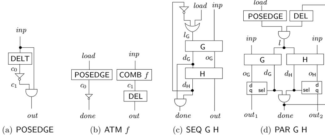
Figure 2.10: Implementation of composite devices.
