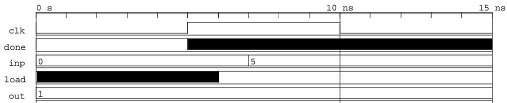
Figure 4.4: Undefined values on the simulation of factorial.
