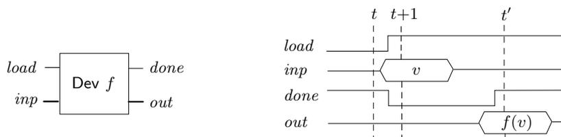
Figure 2.8: Handshaking device.
