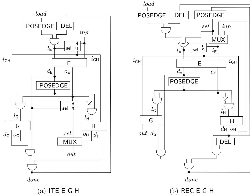
Figure 2.11: The conditional and the recursive constructors.
