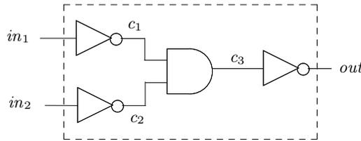
$$\vdash \text{OR\_IMP}(in_1, in_2, out) = \exists c_1\ c_2\ c_3. \text{NOT}(in_1, c_1) \wedge \text{NOT}(in_2, c_2) \wedge \text{AND}(c_1, c_2, c_3) \wedge \text{NOT}(c_3, out)$$
