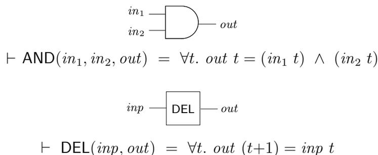
Figure 2.3: Primitive components in HOL.
