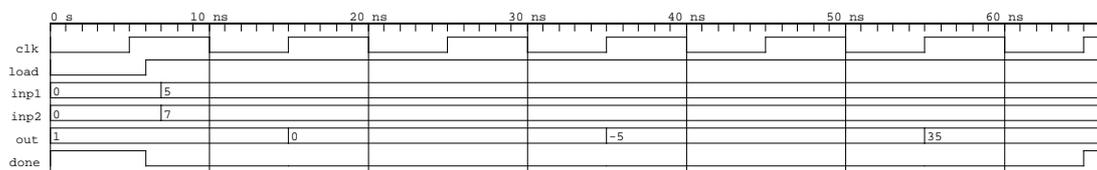
Figure 5.3: Simulation of the ARM6 Booth's algorithm computing  $5 \times 7$ .
