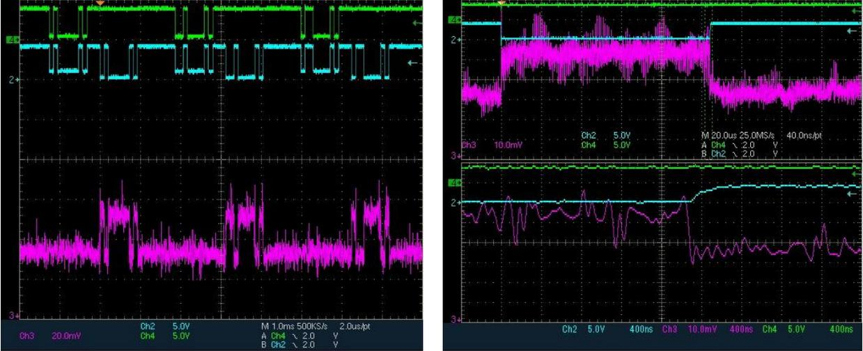
Figure 36. Power trace acquired with a passive probe, 500KS/s and 25MS/s rates
