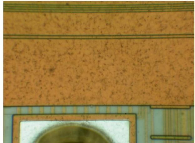
Figure 13. Nothing can be seen under the top metal layer on Microchip PIC16F877A microcontroller [37] as the layers inside the chip were planarised during fabrication. 500× magnification
