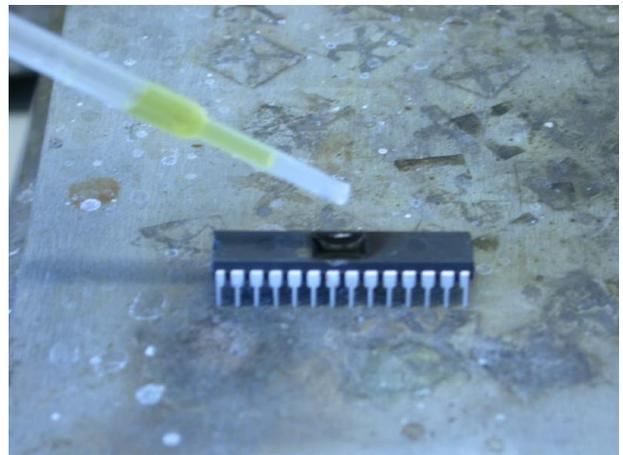
Figure 51. Manual decapsulation tools and dropping the fuming nitric acid into the pre-milled hole
