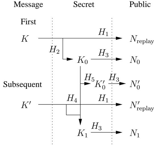
Figure 6.1: Cryptographic key derivation in an *fs-mix*.
