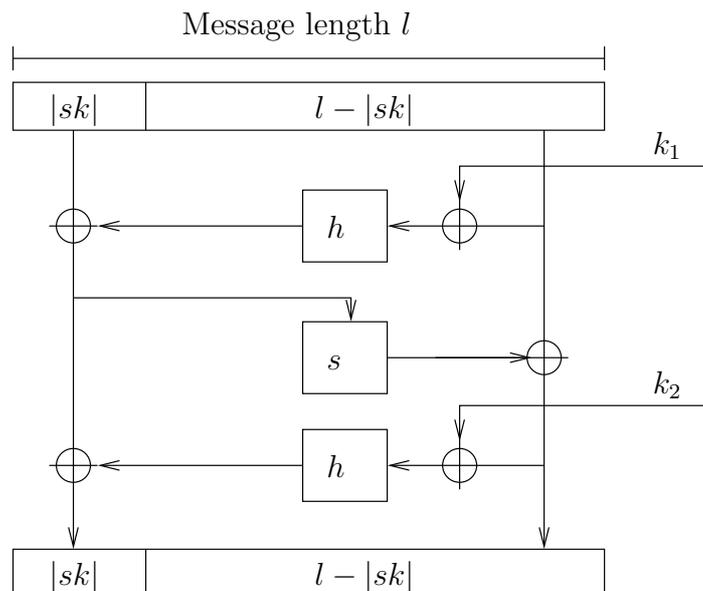
Figure 3.1: The structure of the BEAR block cipher
