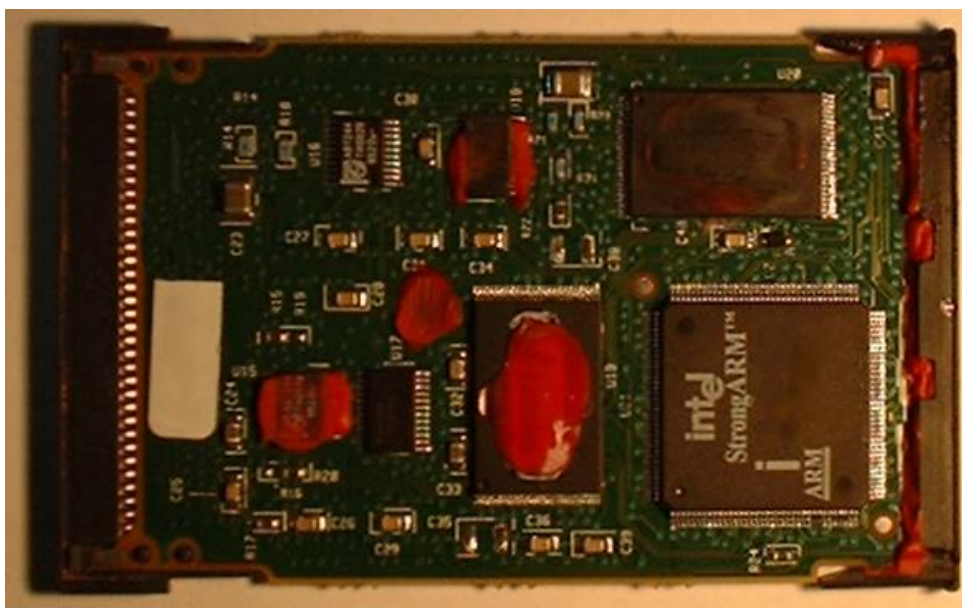
Figure 3: A Luna CA 3 token disassembled
