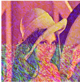
Figure 7.1: A single bit was artificially flipped half-way through the file produced by a GELIC encoder. The disastrous effect of the error on the decoded image can be clearly seen.
