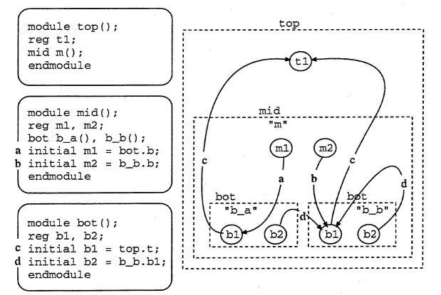
a) a downward reference by module type name, b) a downward reference by instance name, c) an upward reference by module type name, which is also a top-level reference and d) an upward reference by instance name.
