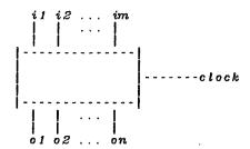
Suppose this device also has some internal registers x1, ..., xp, and that it behaves like a sequential machine as follows:
