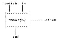
Here the input lines are *switch* and in, the only output line is *out* and the only state variable is n. The name of the device is COUNT; we write COUNT(n) to show that the behaviour (to be described) depends on n (actually COUNT would be an OL constant of type num->dev). Suppose the behaviour of COUNT is informally specified by:
