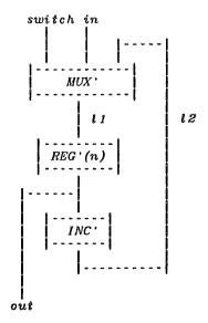
This device is built from components similar to MUX, REG(n) and INC as described above, except that the line names have been changed. The multiplexer MUX' is like MUX except that it has lines in, i2, i1 instead of i1, i2, o respectively. The need to rename lines motivates the following kind of term:
