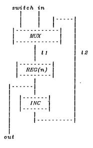
Note that MUX, REG and INC (as defined by behaviour equations above) have different line names to those in this diagram. For example, MUX was defined to have lines i1, i2 and o instead of in, i2 and i1. This illustrates our convention of using the names in diagrams to indicate renaming.
