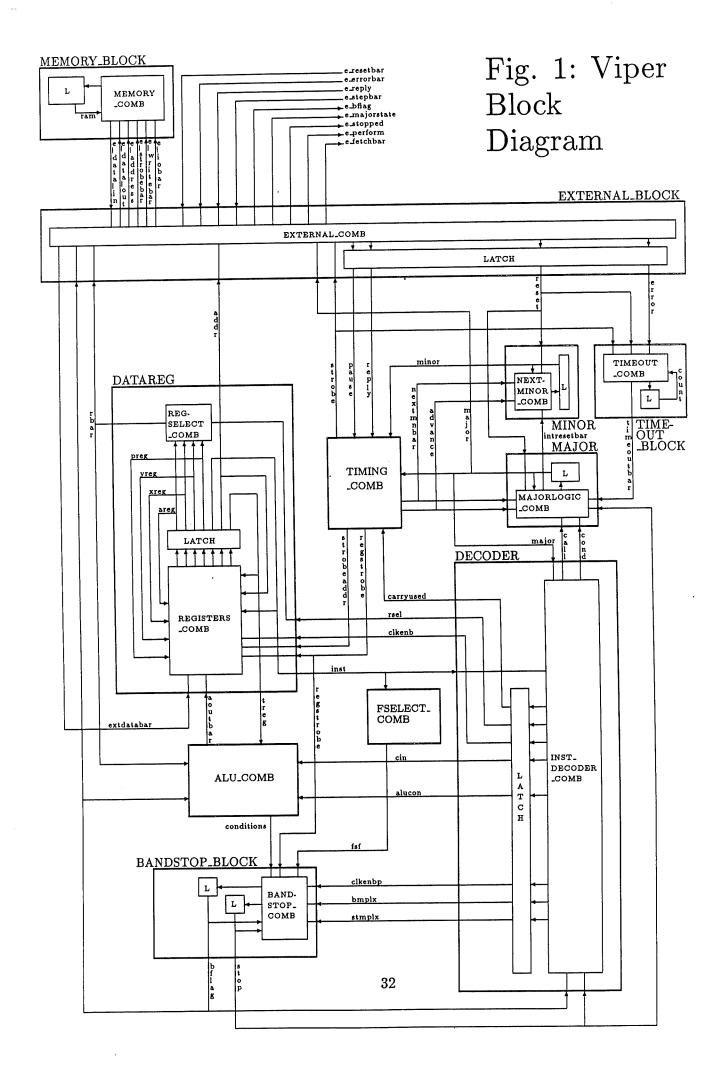
data (e\_data\_in); aoutbar, the 32-bit data output of the arithmetic-logic unit; clkenb, a line from the decoder controlling when and which registers of dataged are to be loaded with new values; and finally, two boolean timing values, regstrobe and strobeaddr, from the timing block, which respectively indicate the stability of an operation, and when the address latch should be loaded.
