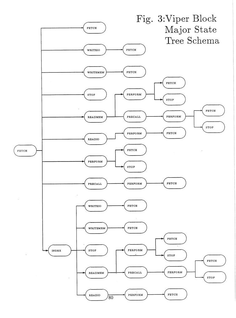
The bolder lines in the figure are path *schemata*, e.g. the collective thirty-or-so paths which follow the pattern of major states shown and contain the PERFORM ALU state. Of these, five or so in each path schema admit the possibility of stopping – e.g. the add-overflow case. The stopping cases are also represented collectively by a bolder line.
