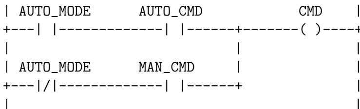
Where `--| |--` is a normally-open contact, `--| /|--` is a normally closed contact, and `--( )--` is a relay coil.
