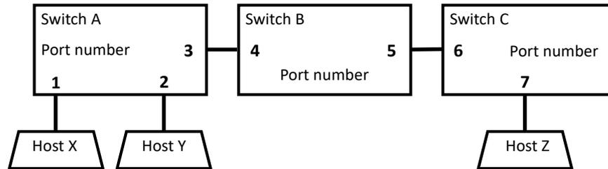
Assuming all switches start with empty switch-forwarding tables; Host X (with physical address X) sends a packet destined for Host Z. Enumerate in the style below, all packets sent across the network until the message arrives at Host Z. You may assume packet-processing, latency and transmission time are negligible. Additionally, indicate packets transmitted simultaneously. [5 marks]
