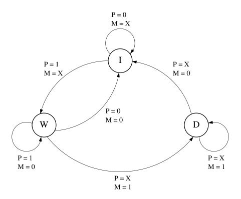
and the state assignment I = [00], W = [01] and D = [10]. Note that state =  $[Q_1Q_2]$  where  $Q_n$  is the output flop flip-flop n.
