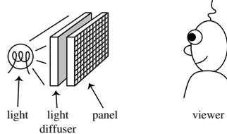
The inventor has recently found that he can make the special ink in *any* colour he likes, but that each panel can be tinted with only one of these colours. He proposes to use three inks in three panels to make a 24-bit colour display: a red-tinted panel, a green-tinted panel and a blue-tinted panel will be stacked up to make a full-colour display (see picture). A value of  $(0, 0, 0)$  will thus be white (transparent),  $(255, 0, 0)$  red and  $(255, 255, 255)$  black.
