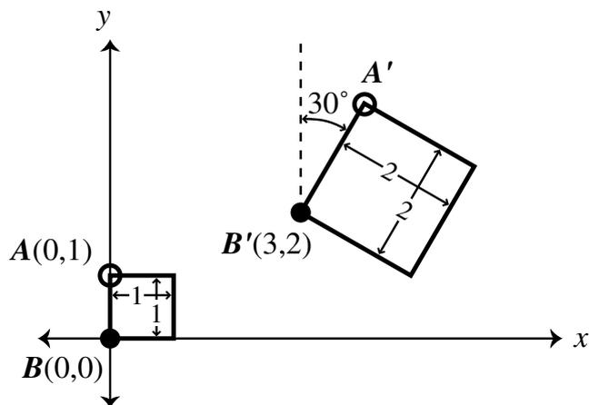
The above diagram shows a complicated 2D transformation applied to a unit square. The overall transformation can be described in terms of a number of simpler transformations. Describe each of these simple transformations and give a matrix representation of each using homogeneous coordinates. [6 marks]
