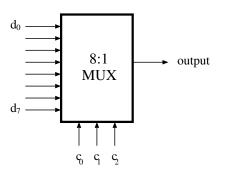
Give a circuit which implements this 8:1 multiplexer using only NAND gates. [10 marks]
