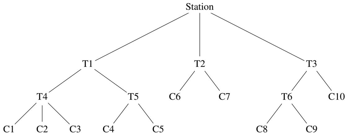
Nodes C1 to C10 are consumers; nodes T1 to T6 are transformers. Each consumer has a direct connection to only one transformer. Sometimes a transformer may malfunction or need to be taken out of service temporarily.
