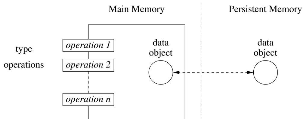
The figure illustrates an object model which is used in a concurrent software system. We are concerned with how to implement atomic operations in the presence of concurrency and crashes.
