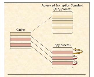
Figure 1. In a Prime+Probe attack, a spy process probes the cache by monitoring timing of accesses to its own memory. As the target process encrypts, it evicts portions of the attacker's memory from the cache, resulting in longer access times. The access times for the individual regions of the attacker's memory correspond to which tables the encryption process accessed, and thus the target's key.
