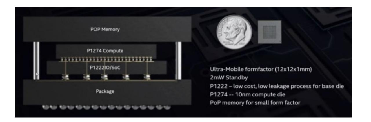
P1274 = 10nm process, P1222 is 22nm FinFET low power (low leakage current) "Foveros" is the 3D face-to-face chip stacking technology, microbumps + Through Silicon Vias (**TSVs**) POP = standard stacked Package-on-Package memory
