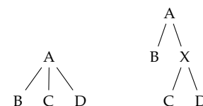
Figure 3: Partial derivations from 2 weakly equivalent context free grammars: the second grammar in Chomsky Normal Form
