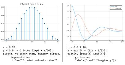
Function plot expects a vectors of x coordinates, and a vector or matrix of y coordinates, one column per curve. Use plot! to add additional curves with independent x coordinates.
